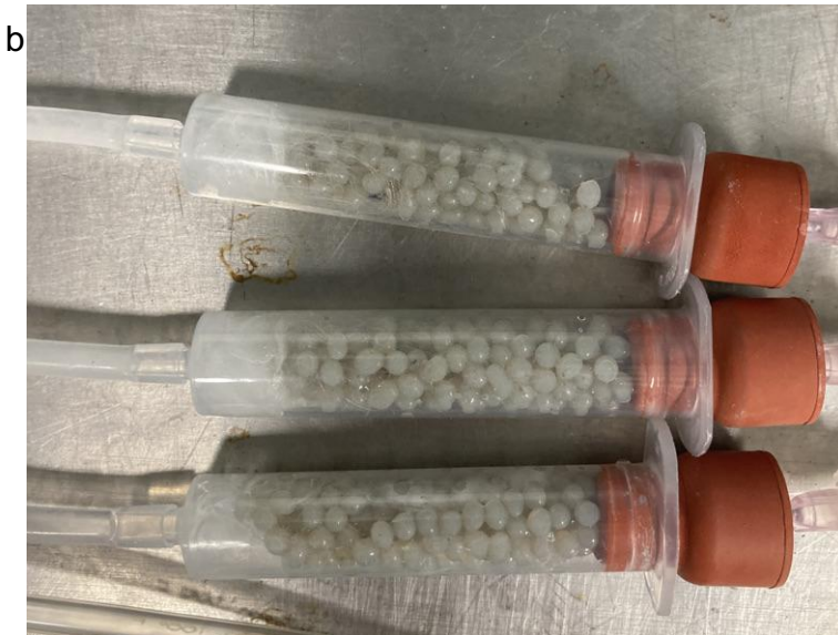
22 Figure S2. Photos of (a) the three-stage system of reactors used to assess bead integrity, with a close-up 23 (b) of alginate beads in the 7-mL flow-through reactor. Data collection from the first and third stages 24 included intact bead count, encapsulated biomass concentration as protein, and gas production.
