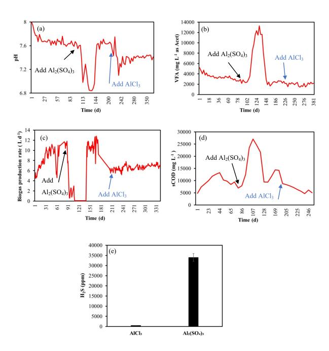
Figure S1. (a) pH, (b) VFA, (c) biogas production rate, and (d) sCOD profiles for the 1:1 PS-to-WAS dry mass blending ratio sludge spiked with high  $Al^{3+}$  dose using two different  $Al^{3+}$ -based coagulants; (e)  $H_2S$  concentration detected in biogas on day 100 and 290 with different  $Al^{3+}$ -based coagulants.
