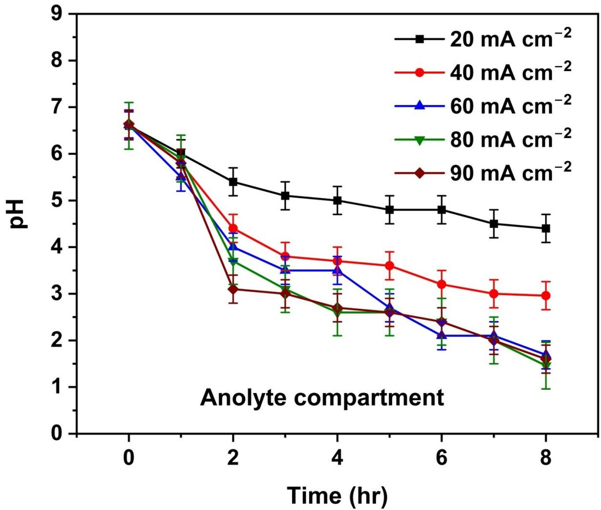
Fig. 8 (a). pH value of SWW at AE tank
