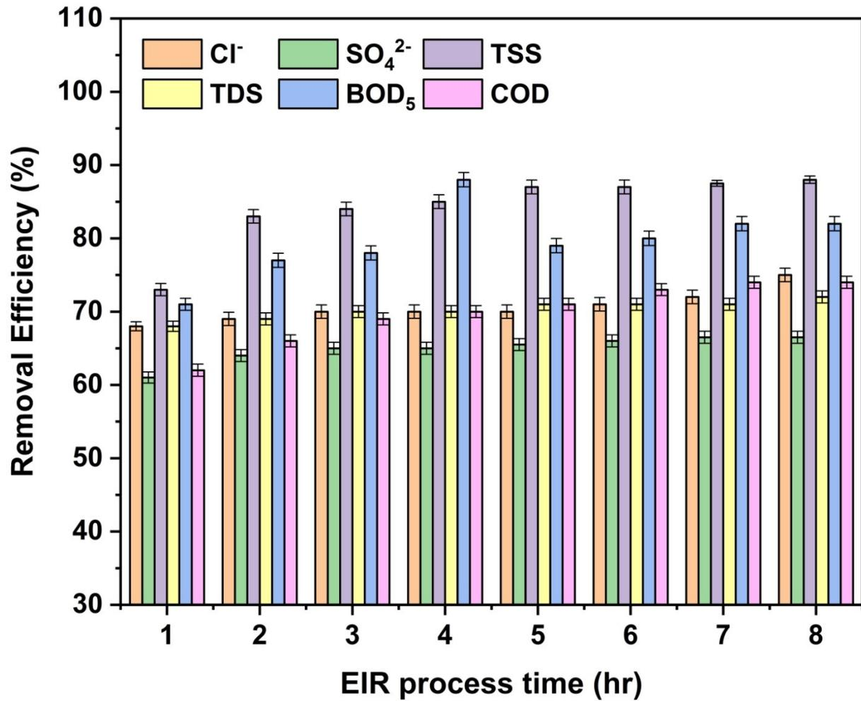
Fig. 2: Effectiveness of time in the EIR process influences the removal efficiencies of pollutants under 1: 1 (v/v) ratio of effluent at the anolyte and catholyte tank respectively, applied current density at 40 mA cm<sup>-2</sup>. The error bars in the results indicate a deviation of  $\pm 1$  standard deviation from the mean of triplicate data.
