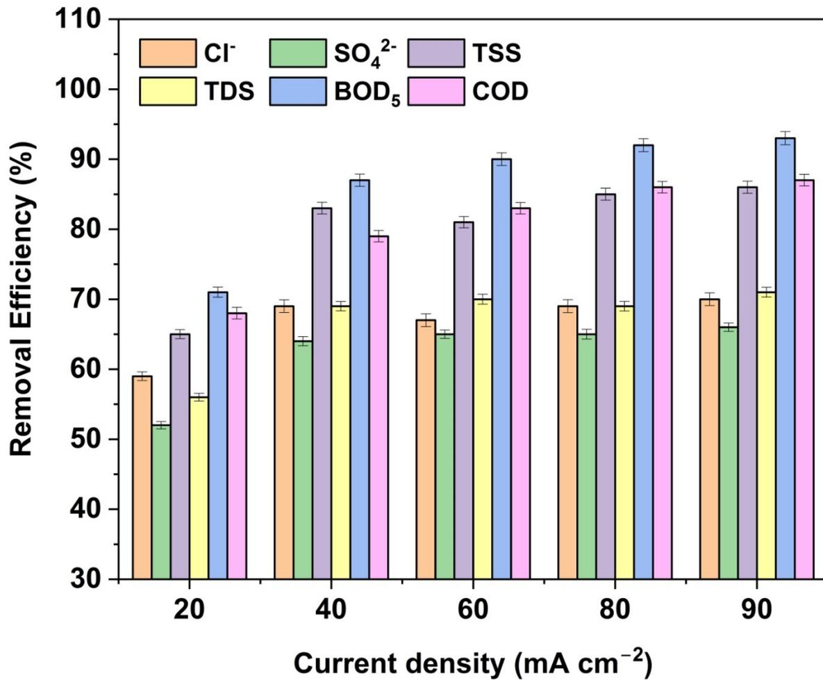
Fig. 5: Varying the CD impacts the efficiency of removing pollutants under 1: 1 (v / v) volume ratio of SWW flow at the anolyte and catholyte tank with respect to optimum time (2hours). The error bars in the results represent a deviation of  $\pm 1$  standard deviation from the mean of triplicate data.
