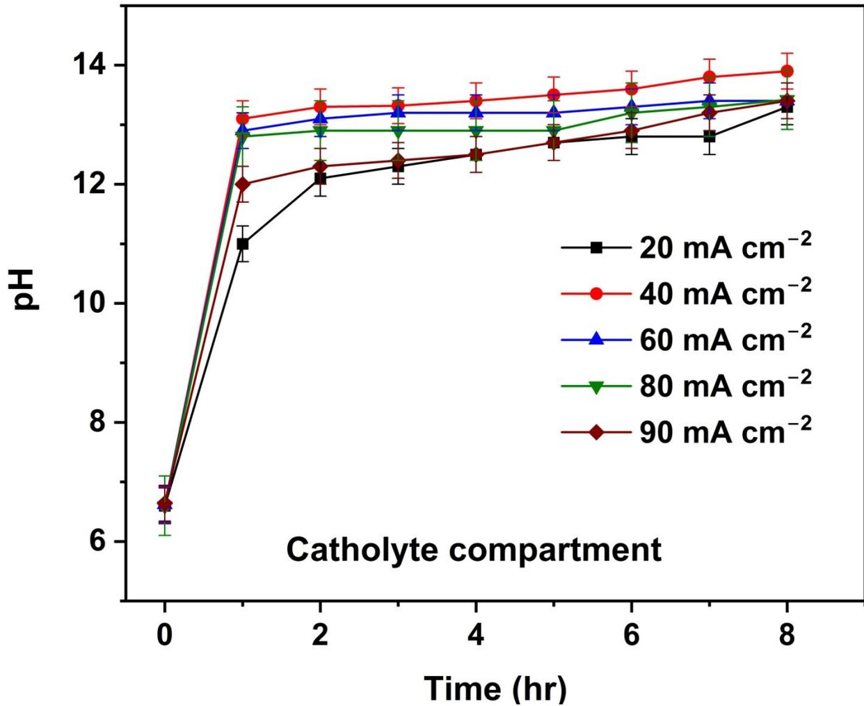
Fig. 8 (b) pH value of SWW at CE tank
