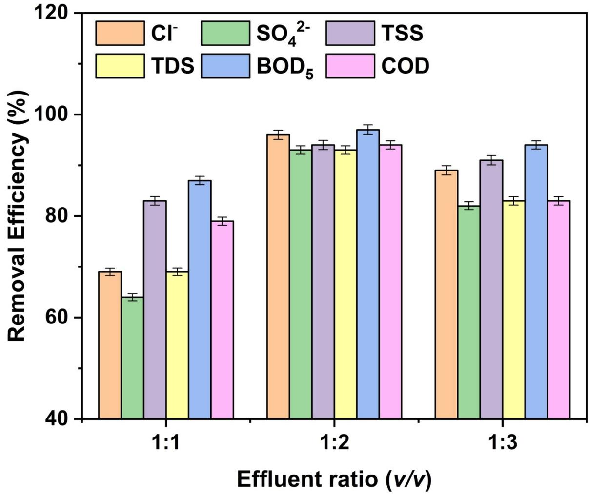
Fig. 9 Removal of effluent efficiency vs various ratio (v / v) of SWW at AE (36 ml / min) & CE tank (15 ml / min) at optimized CD (40 mA cm<sup>-2</sup>) and time (2hours) at the recirculation flow rate. The error bars in the results represent a deviation of ±1 standard deviation from the mean of triplicate data.
