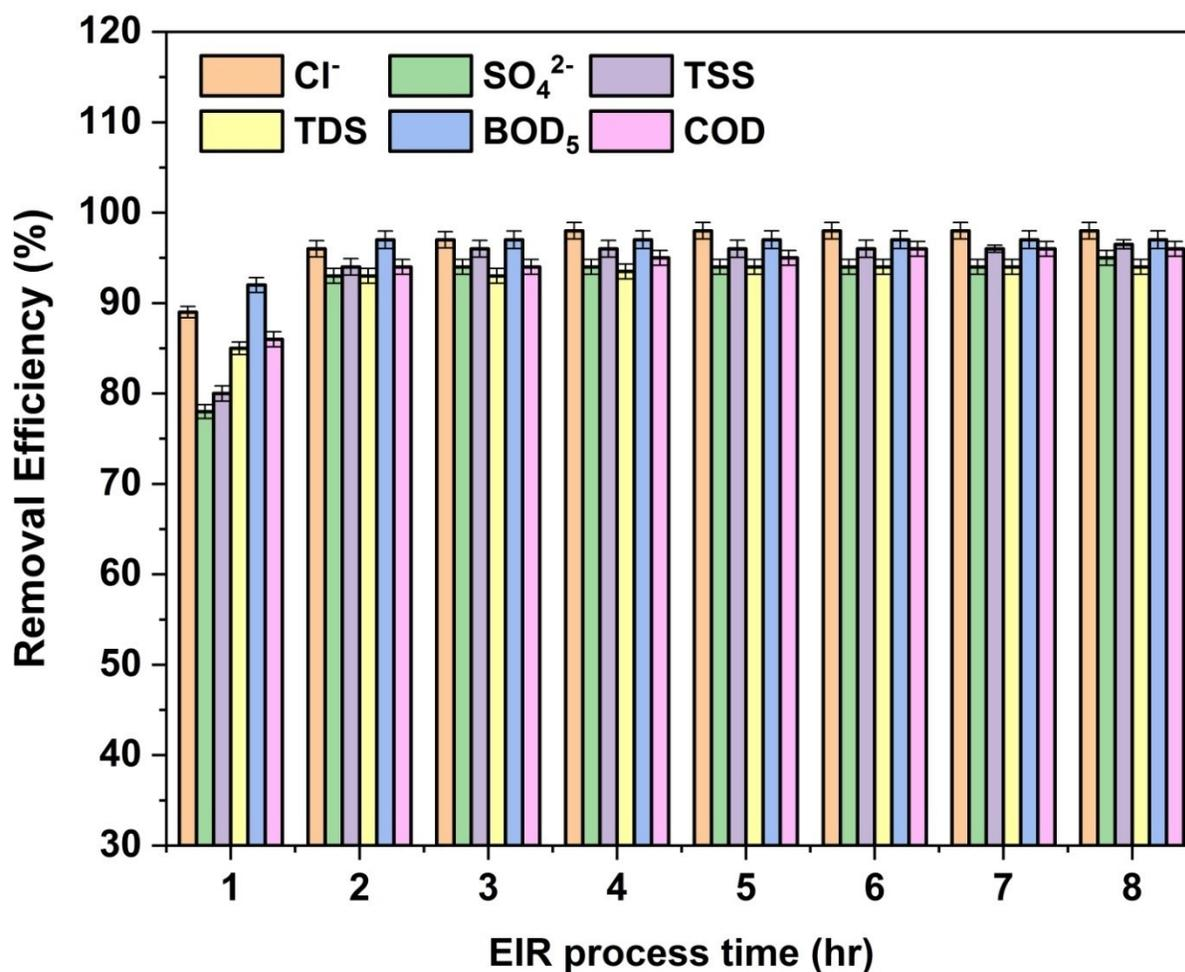
Fig. 3: Effectiveness of time in the EIR process influences the removal efficiencies of pollutants under 1: 2 (v/v) ratio of effluent at the anolyte and catholyte tank respectively, applied current density at 40 mA cm<sup>-2</sup>. The error bars in the results indicate a deviation of ±1 standard deviation from the mean of triplicate data.
