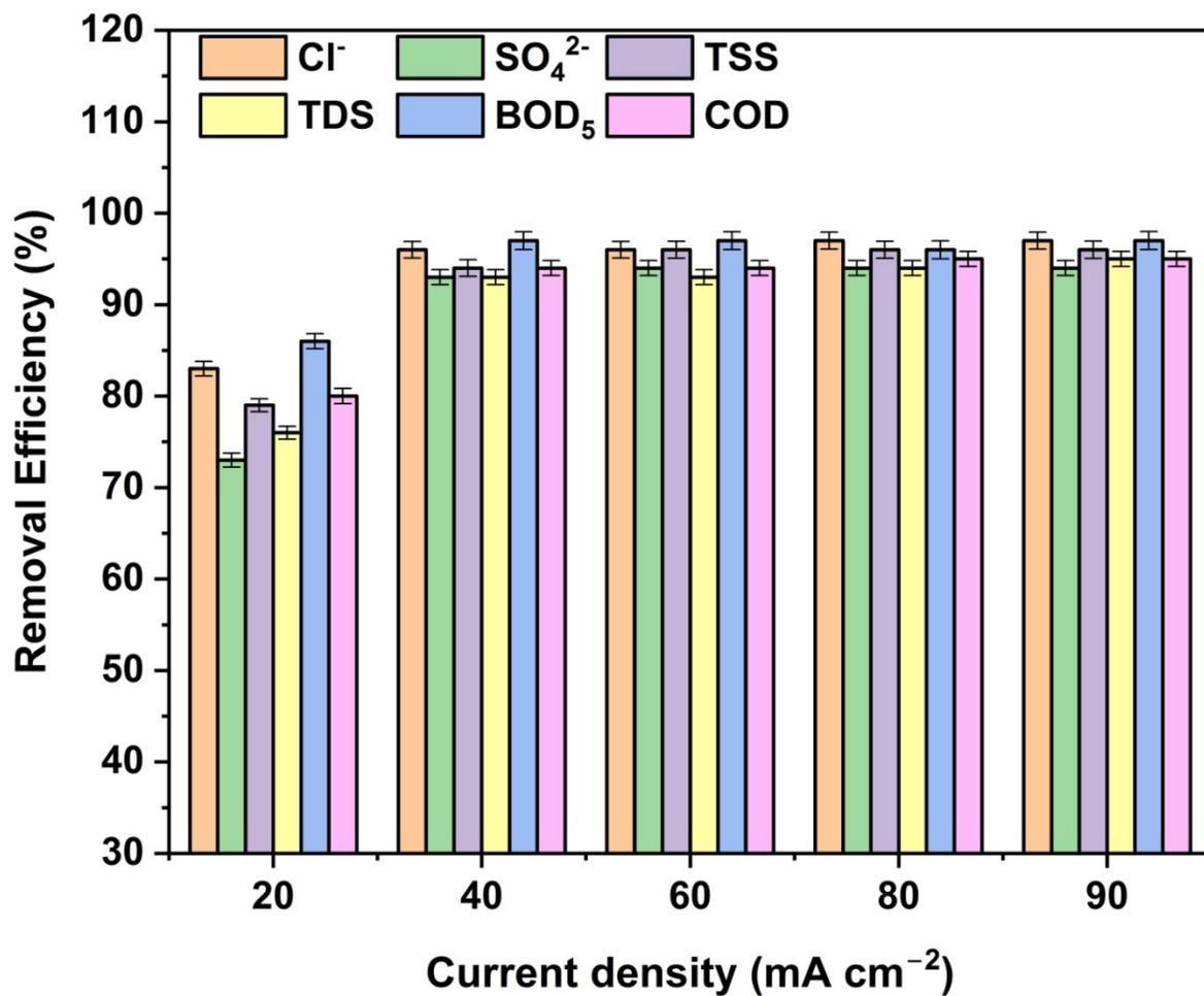
Fig. 6: Varying the CD impacts the efficiency of removing pollutants under 1: 2 (v / v) volume ratio of SWW flow at the anolyte and catholyte tank with respect to optimum time (2hours). The error bars in the results represent a deviation of  $\pm 1$  standard deviation from the mean of triplicate data.
