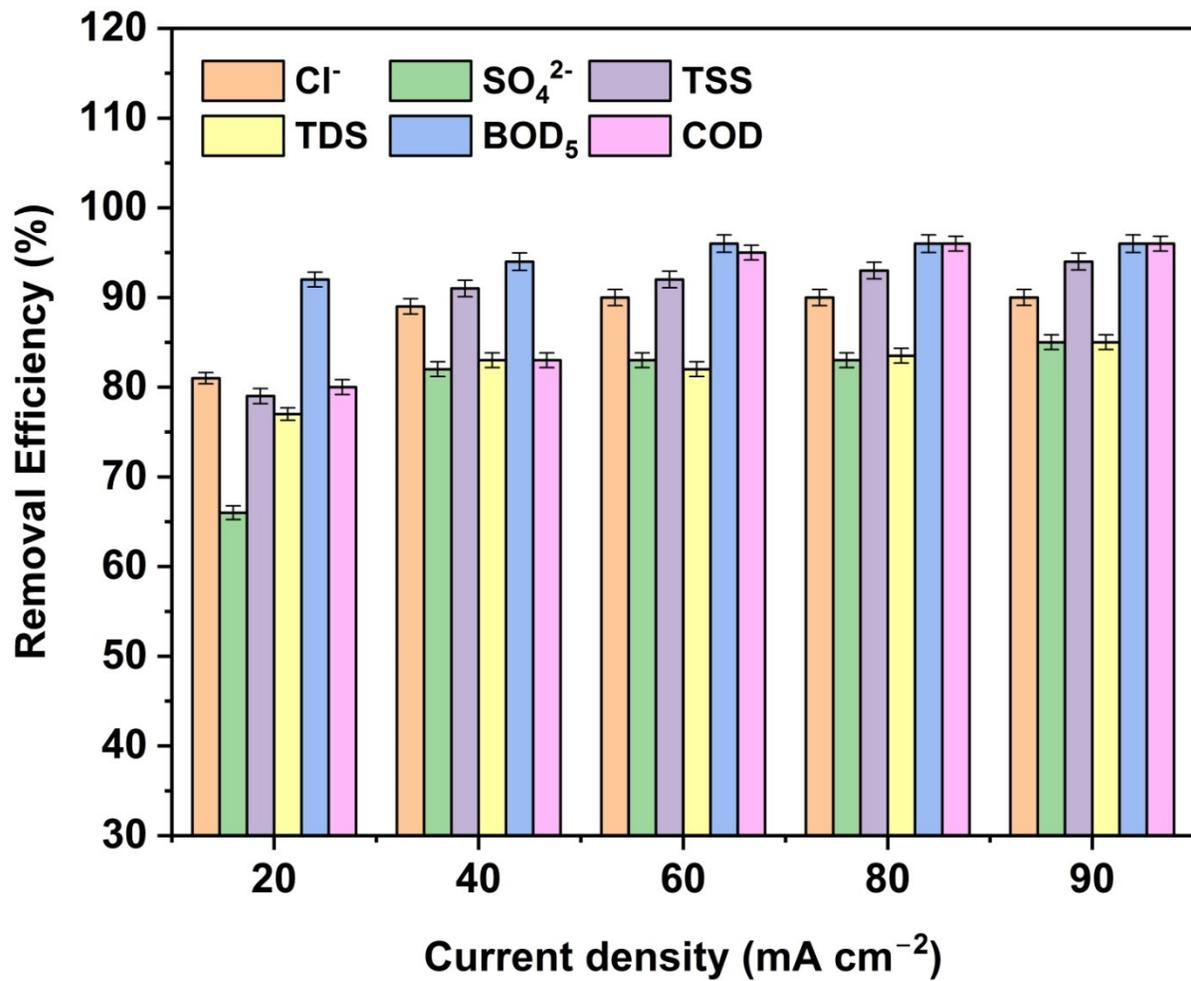
Fig. 7: Varying the current density (CD) impacts the efficiency of removing pollutants under 1: 3 (v / v) ratio of effluent flow at the anolyte and catholyte tank with respect to optimum time (2hours). The error bars in the results represent a deviation of  $\pm 1$  standard deviation from the mean of triplicate data.
