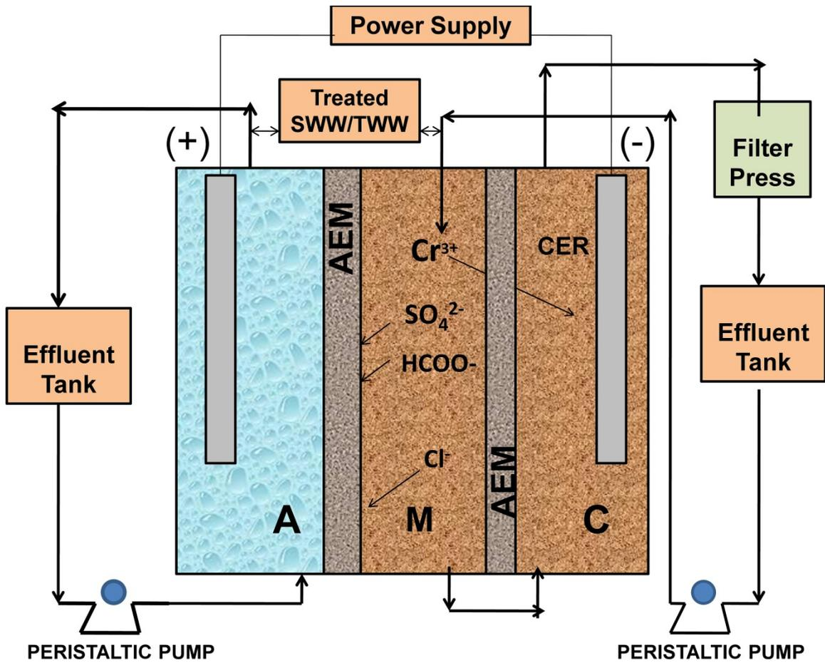
**Fig. 1:** Schematic representation of EIR setup of SWW / TWW effluent treatment process.
