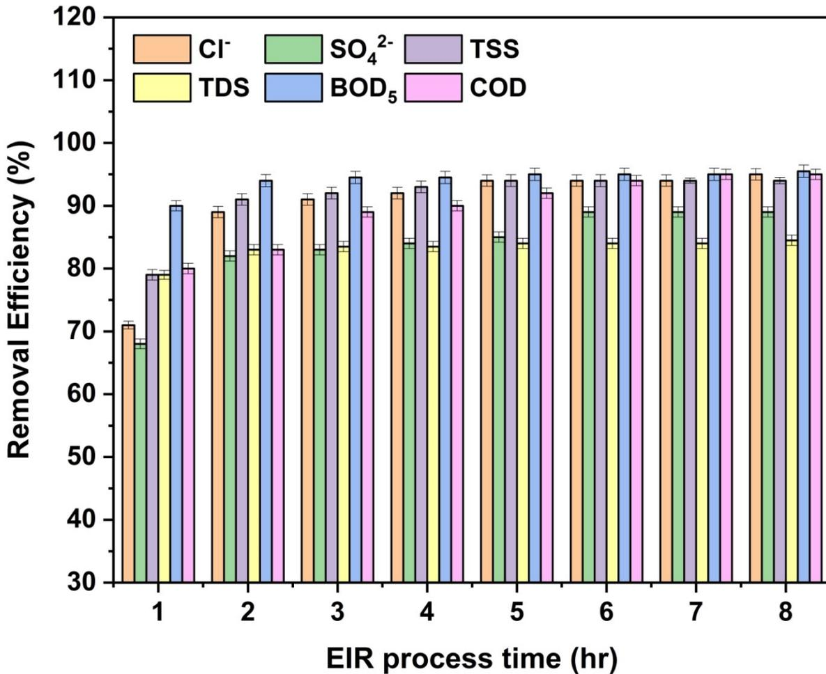
Fig. 4: Effectiveness of time in the EIR process influences the removal efficiencies of pollutants under 1: 3 (v/v) ratio of effluent at the anolyte and catholyte tank respectively, applied current density at 40 mA cm<sup>-2</sup>. The error bars in the results indicate a deviation of ±1 standard deviation from the mean of triplicate data.
