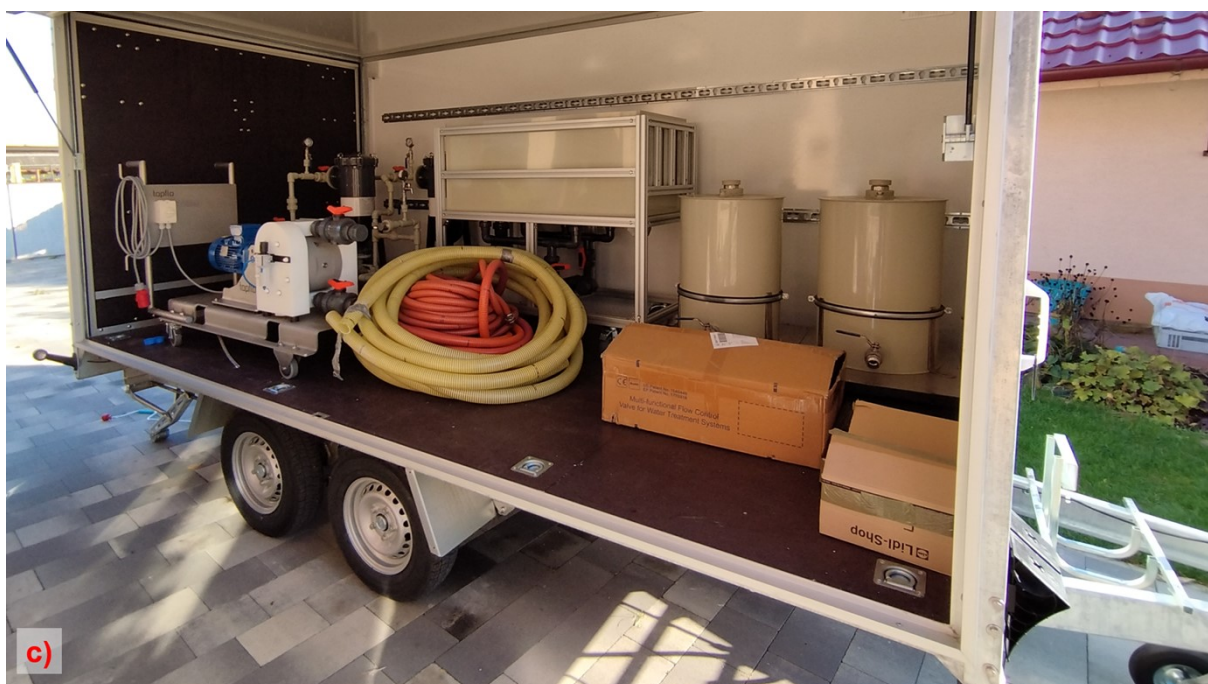
Figure S1: a) Actual photograph of the operational electrochemical field setup, b) 3D model of mobile field EC unit and c) actual photograph of the mobile field EC unit.
