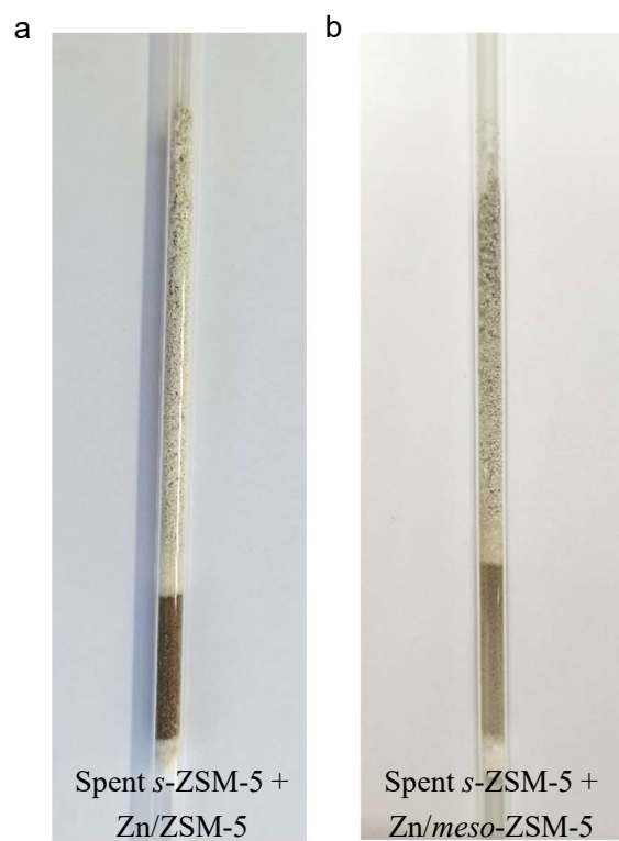
Figure S4. Photographs of the spent (a) s -ZSM-5+Zn/ZSM-5, (b) s -ZSM-5+Zn/ meso -ZSM-5. Reaction conditions: the mixture of 500 mg of PE and 100 mg of s -ZSM-5 in the first bed, 400 mg of catalyst for aromatization in the second bed, feed gas of 3.3% H 2 /29.7% Ar/67% N 2 , a flow rate of 3 mL/min, 400 °C, 4 h.
