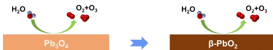
Figure S12. The schematic illustration of the complete reconstruction of \text{Pb}_3\text{O}_4 before and after the EOP process at the constant current condition of 1.0 \text{ A/cm}^2 (anode potential was between 2.40 to 2.45 V vs.RHE).
