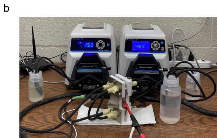
Fig. S25. Working principles of \text{NO}_3^- concentrating and the experimental electrodedialysis system. (a) Schematic illustrating the working principles of \text{NO}_3^- concentrating via electrodedialysis with one electrodedialysis pair (CEM | diluate solution | AEM | concentrate solution), and one additional CEM (part of background cell). (b) Photo of our experimental electrodedialysis system in operation encompassing one electrodedialysis cell, two peristaltic pumps, and three solution containers (diluate, concentrate, and electrode solutions).
