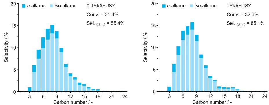
**Figure S6.** Hydrocracking of PE over Pt on  $\gamma$ -Al<sub>2</sub>O<sub>3</sub> with different loading. Reaction conditions: PE, 4.0 g, 280 °C, 3 MPa H<sub>2</sub>, 3 h, for 0.1Pt/A + USY the catalyst weight is 0.2 g + 0.2 g, for 1Pt/A + USY the catalyst weight is 0.02 g + 0.2 g.
