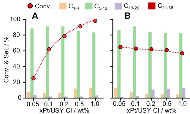
**Figure S4.** Hydrocracking of PE over Pt/USY catalysts with different Pt loading. Reaction conditions: A) PE, 4.0 g, catalyst, 0.2 g, 280 °C, 3 MPa H<sub>2</sub>, 3 h; B) PE, 4.0 g, catalyst, from 0.4 g to 0.02 g to keep Pt usage at 0.2 mg, 280 °C, 3 MPa H<sub>2</sub>, 3 h.
