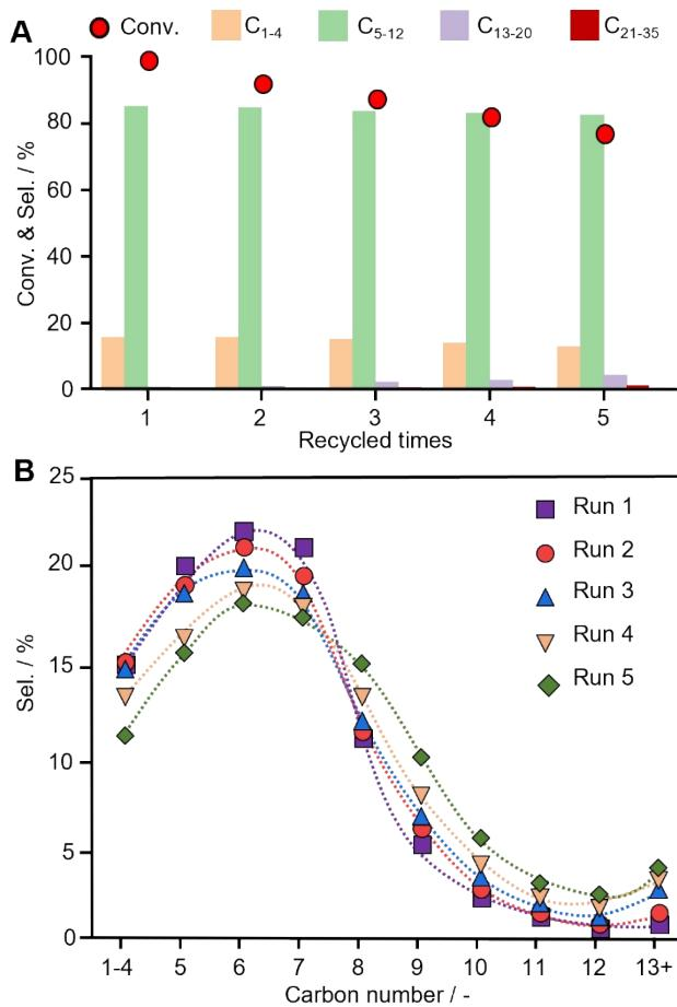
**Figure S12.** Reusability test of 0.1Pt/USY-CI catalyst. A) Catalytic performance and B) product distribution over run times. Reaction conditions: PE, 4.0 g, catalyst (1Pt/USY-CI), 0.4 g, 280 °C, 3 MPa H<sub>2</sub>, 6 h.
