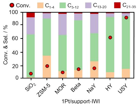
**Figure S3.** Hydrocracking of PE over 1wt% Pt on different supports. Reaction conditions: PE, 4.0 g, catalyst, 0.2 g, 280 °C, 3 MPa H<sub>2</sub>, 3 h.
