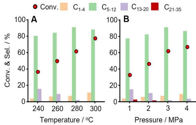
**Figure S2.** Hydrocracking of PE at different temperature and H<sub>2</sub> pressure over 0.1Pt/USY-CI. Reaction conditions:
