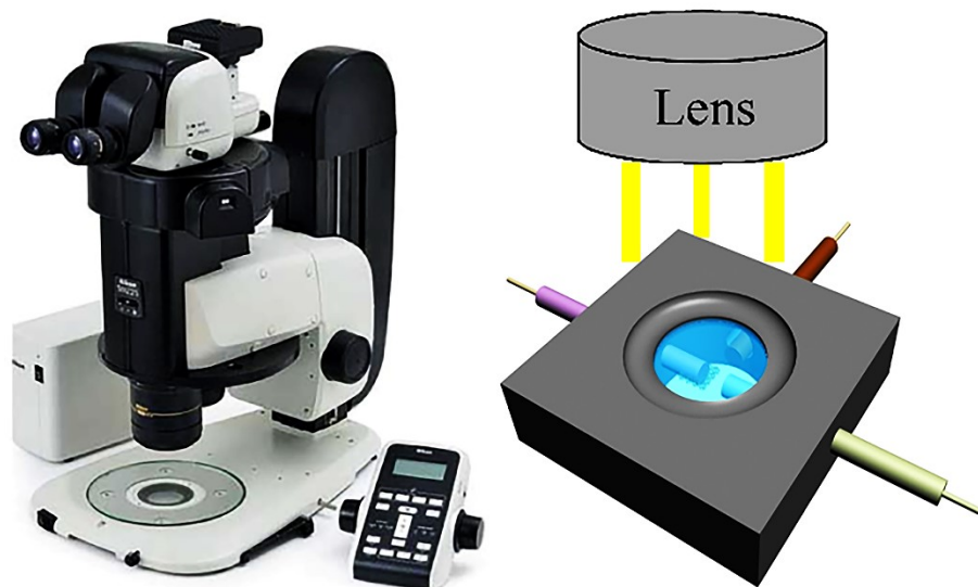
Figure S12. Schematic representation of the operando optical microscopy of gas bubbles using a home-made three-electrode electrochemical cell with a transparent window.
