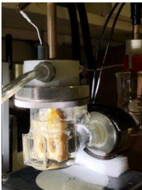
Figure S1. Photograph of the H-cell setup showing the cell holder made from PEEK. Exposed illuminated area is 0.28 \text{ cm}^2 corresponding to a circular area with a diameter of 6 mm.
