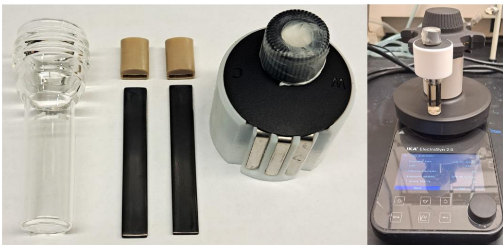
Fig. S1. Photographs of the experimental setup for DC electrolysis using a commercial IKA ElectraSyn 2.0.
