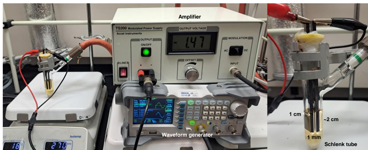
Fig. S2. Photographs of the experimental setup for AC electrolysis consisting of a TS200 amplifier from Accel Instruments and RIGOL DG1062 waveform generator, a Schlenk tube, and two glassy carbon electrodes.
