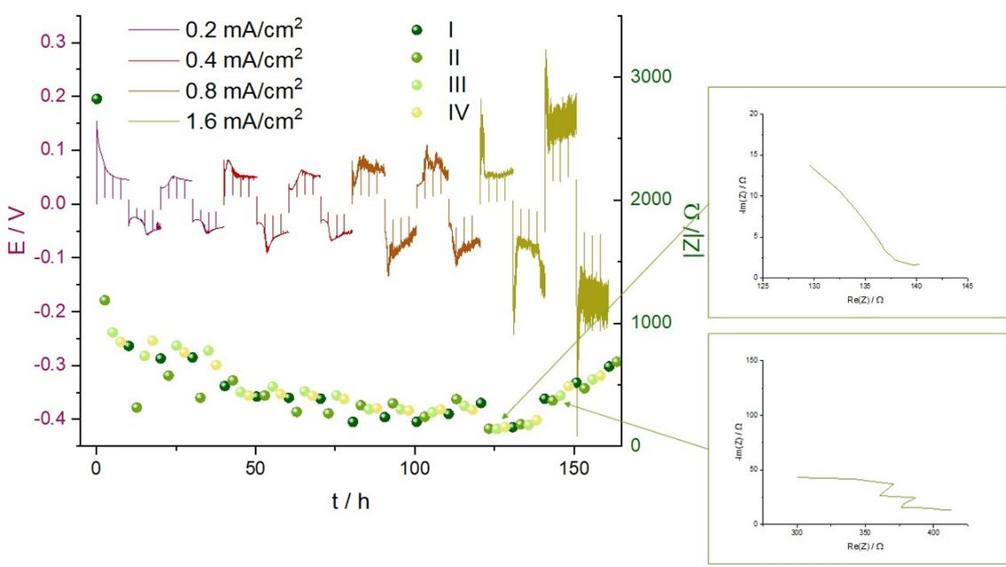
**Figure S3:** voltage trace of galvanostatic cycling for Li-Li symmetric Swagelok cells 1M LiTFSI electrolyte in TEGDME in Ar atmosphere and the corresponding impedance magnitude |Z| at 9 Hz. Inserts are Nyquist plots before and after soft shorting occurs.
