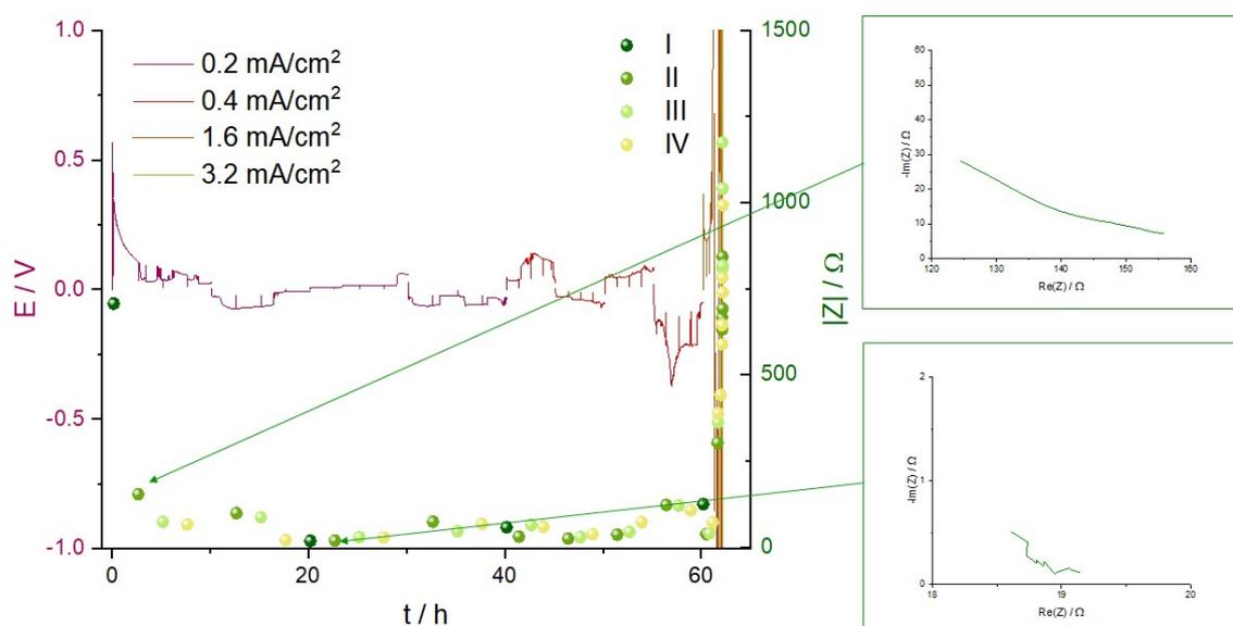
**Figure S6:** voltage trace of galvanostatic cycling for Li-Li symmetric coin cells 1M LiTFSI electrolyte in DMSO prepared in Ar atmosphere and the corresponding impedance magnitude  $|Z|$  at 9 Hz (a) full scale (b) rescaled. Inserts are Nyquist plots before and after soft shorting occurs.
