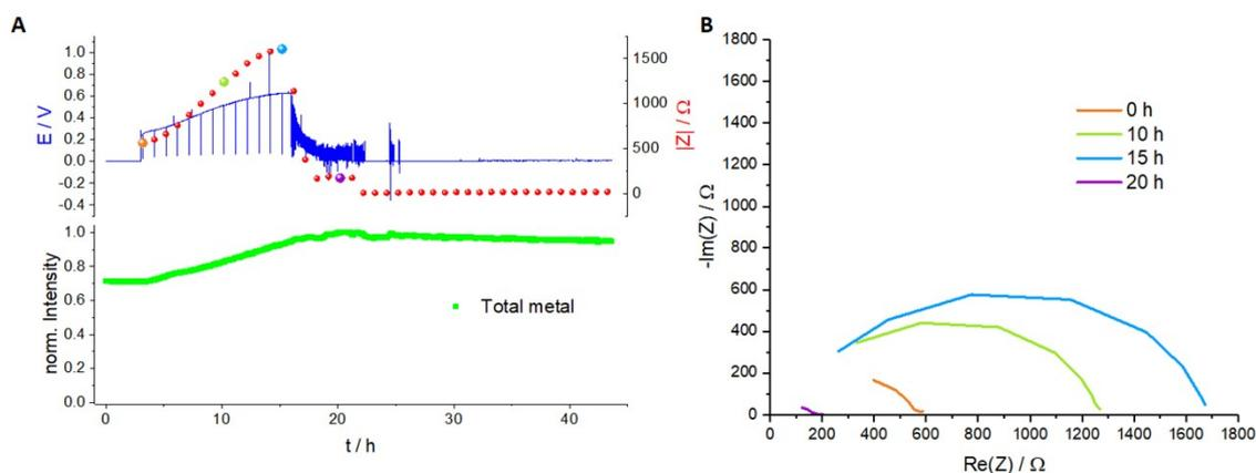
**Figure S8:** Operando NMR spectroscopic measurements of Li metal plating at  $1\text{mA cm}^{-2}$  in symmetrical Li cell with 1 M LiTFSI in TEGDME under  $\text{O}_2$  atmosphere (A) and the Nyquist plots during plating (B).
