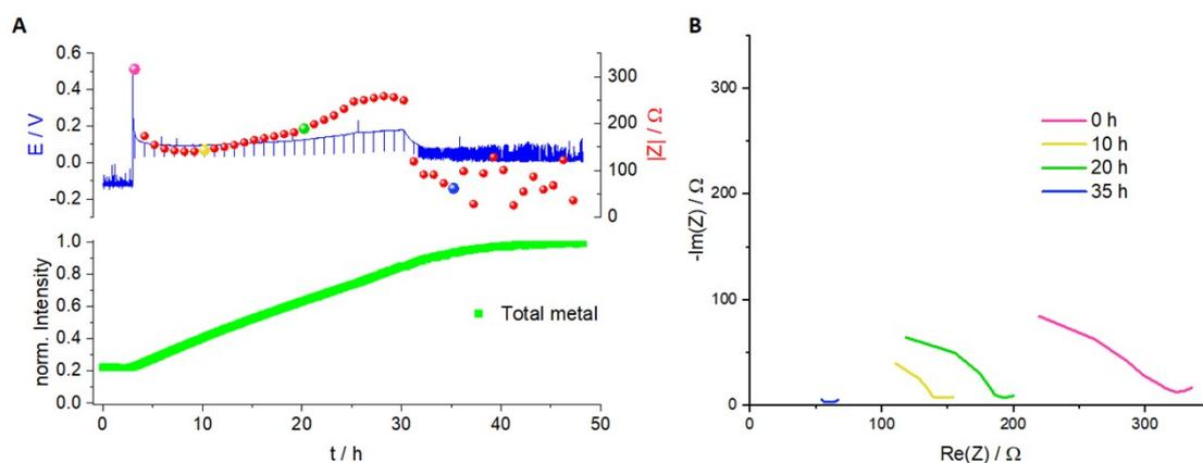
**Figure S7:** Operando NMR spectroscopic measurements of Li metal plating at  $1\text{mA cm}^{-2}$  in symmetrical Li cell with 1 M LiTFSI in DMSO under  $\text{O}_2$  atmosphere (A) and the Nyquist plots during plating (B).
