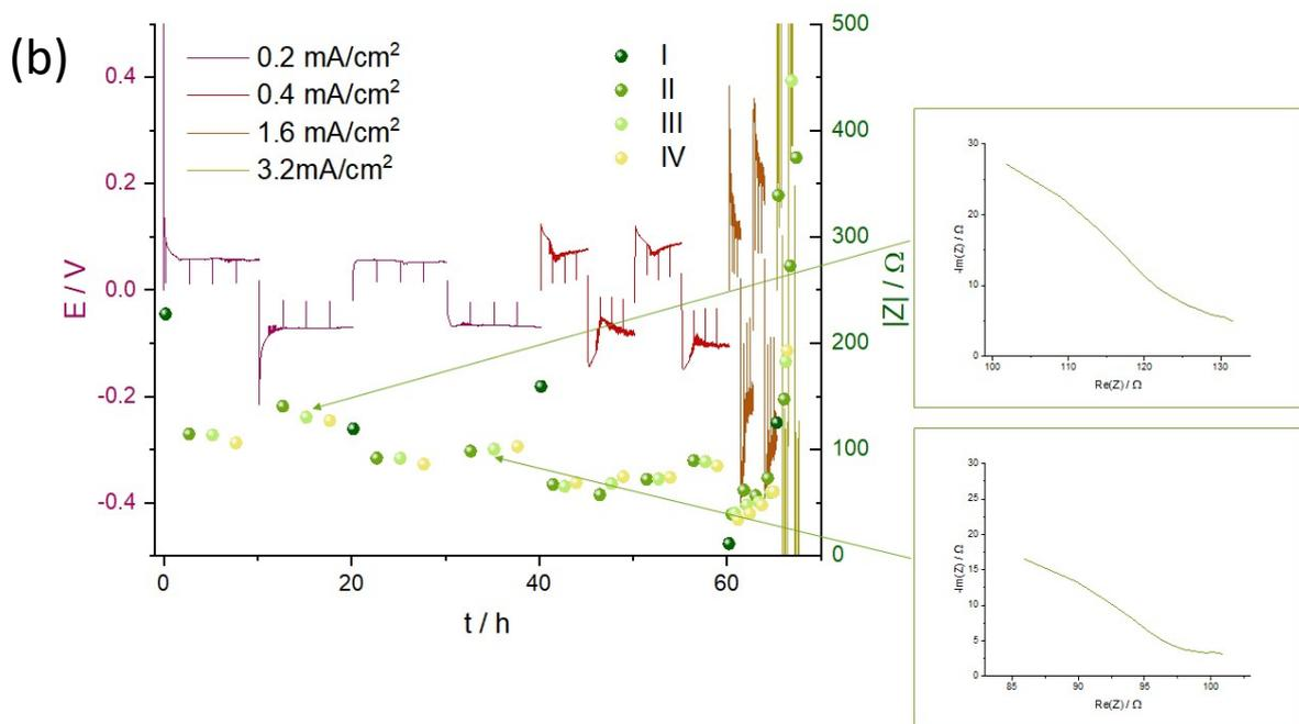
**Figure S5:** voltage trace of galvanostatic cycling for Li-Li symmetric coin cells 1M LiTFSI electrolyte in TEGDME prepared in Ar atmosphere and the corresponding impedance magnitude  $|Z|$  at 9 Hz (A) full scale (B) rescaled. Inserts are Nyquist plots with no clear evidence of soft shorting occurring.
