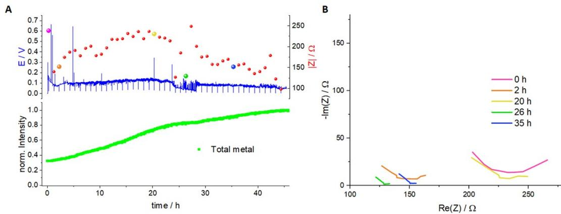
**Figure S9:** Operando NMR spectroscopic measurements of Li metal plating at  $1\text{mA cm}^{-2}$  in symmetrical Li cell with 1 M LiTFSI in TEGDME under Ar atmosphere (A) and the Nyquist plots during plating (B).
