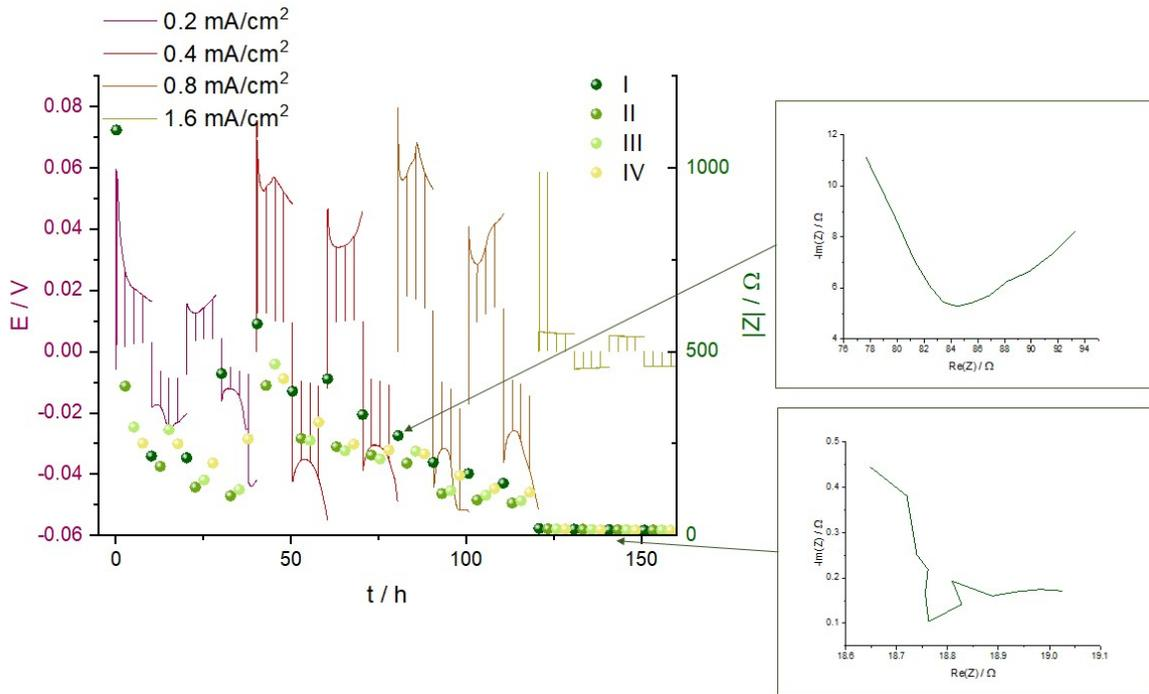
**Figure S2:** voltage trace of galvanostatic cycling for Li-Li symmetric Swagelok cells 1M LiTFSI electrolyte in DMSO in O<sub>2</sub> atmosphere and the corresponding impedance magnitude |Z| at 9 Hz. Inserts are Nyquist plots before and after soft shorting occurs.
