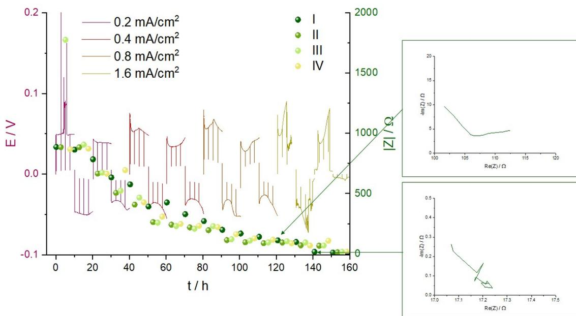
**Figure S4:** voltage trace of galvanostatic cycling for Li-Li symmetric Swagelok cells 1M LiTFSI electrolyte in TEGDME in O<sub>2</sub> atmosphere and the corresponding impedance magnitude  $|Z|$  at 9 Hz. Inserts are Nyquist plots before and after soft shorting occurs.
