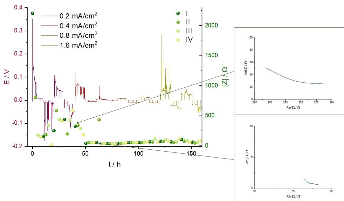
**Figure S1:** voltage trace of galvanostatic cycling for Li-Li symmetric Swagelok cells in 1M LiTFSI electrolyte in DMSO in Ar atmosphere and the corresponding impedance magnitude  $|Z|$  at 9 Hz. Inserts are Nyquist plots before and after soft shorting occurs.
