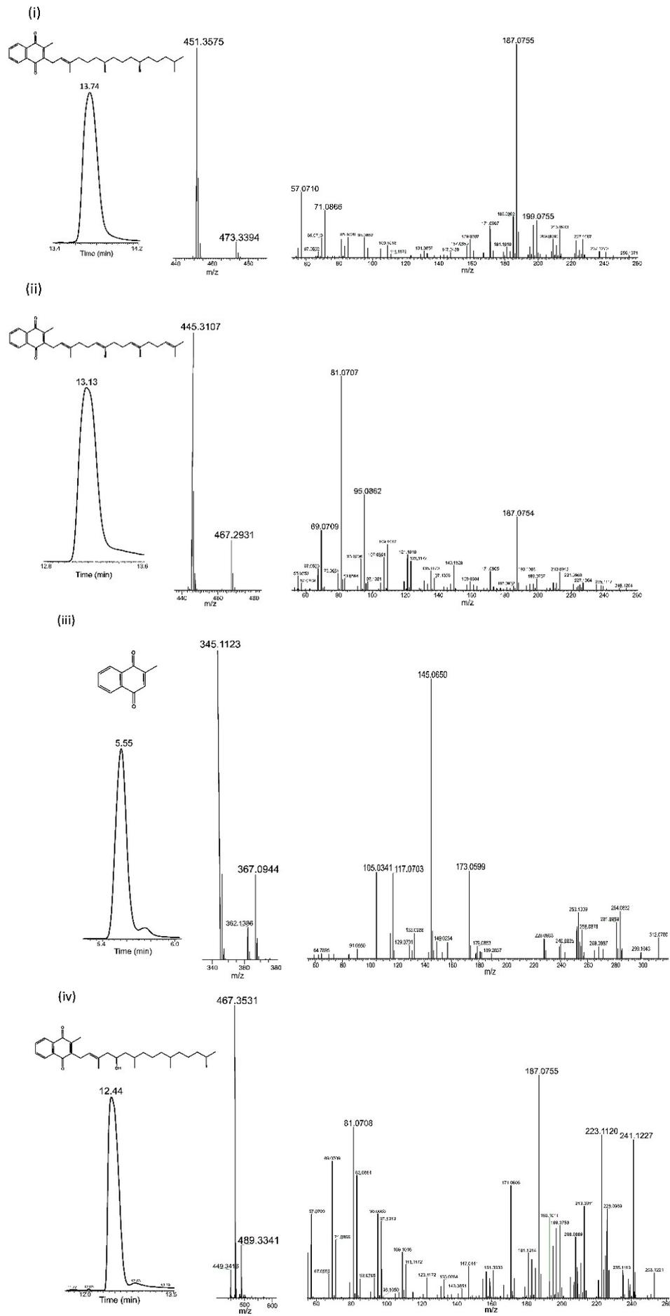
**Figure S 10** LC-ESI-HRMS/MS spectra of vitamin K isoforms in the positive ion mode, showing the retention time (RT) and major detected adducts from MS1 data and fragmentation from MS2 data. (i) Phylloquinone, (ii) Menaquinone (MK-4), (iii) Menadione and (iv) OH-PhQ.
