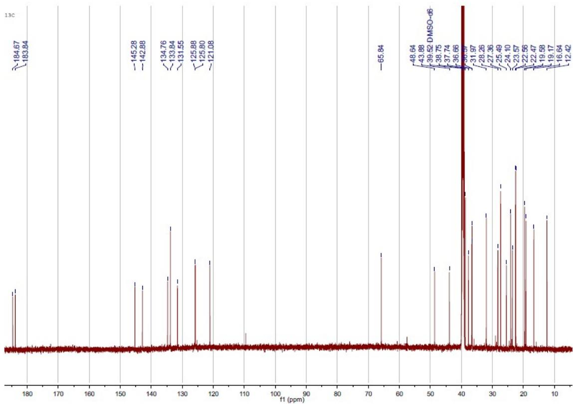
Figure 3  $^{13}\text{C}$  NMR spectrum of 5'-OH-Phylloquinone in DMSO- $d_6$  (600 MHz).
