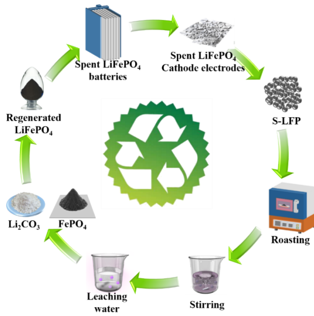
Figure S1. Flow chart of the recovery of spent \text{LiFePO}_4 batteries in this work
