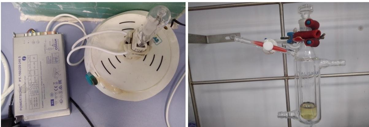
**Figure S1.** Photographs of parts of a custom made photochemical reactor setup used to perform reactions described in this work. Metal halide lamp with a magnetic stirrer and inbuilt fan (left) and a jacketed flask made of Pyrex glass (right) were used.
