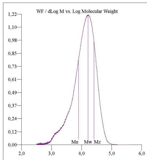
Figure S28: SEC chromatogram after complete devolatilization (absence of volatile cyclics: D3/D4/D5)
