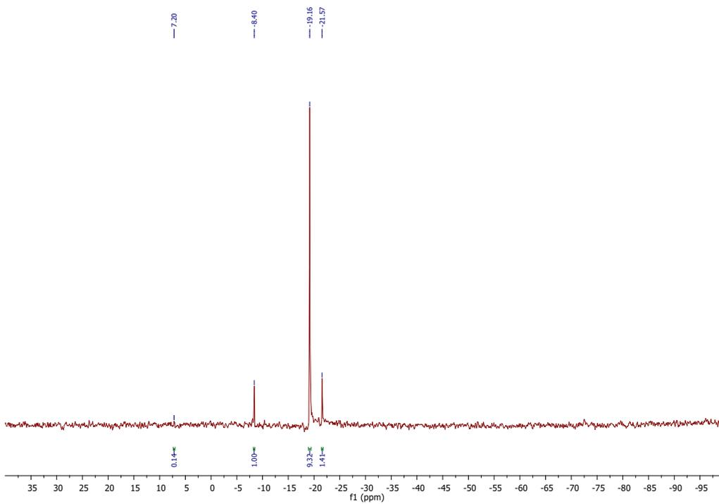
Figure S18:  $^{29}\text{Si}$ -NMR spectrum of depolymerization products of RTV2 + **1** (25°C,  $\text{CDCl}_3$ , 59.6 MHz)
