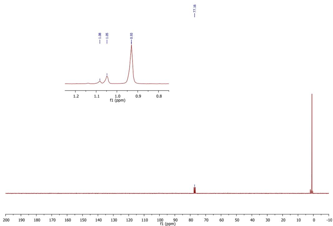
Figure S5:  $^{13}\text{C}$ -NMR spectrum of depolymerization products of silicone oil **1** ( $D_3$ ,  $D_4$ ,  $D_5$ ) (25°C,  $\text{CDCl}_3$ , 75 MHz)
