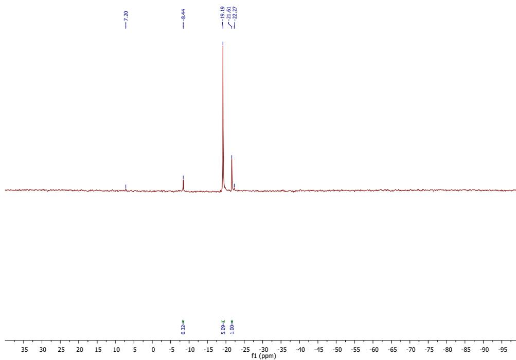
Figure S11:  $^{29}\text{Si}$ -NMR spectrum of depolymerization products of silicone oil **6 + 1** ( $D_3$ ,  $D_4$ ,  $D_5$ ) (25°C,  $\text{CDCl}_3$ , 59.6 MHz)
