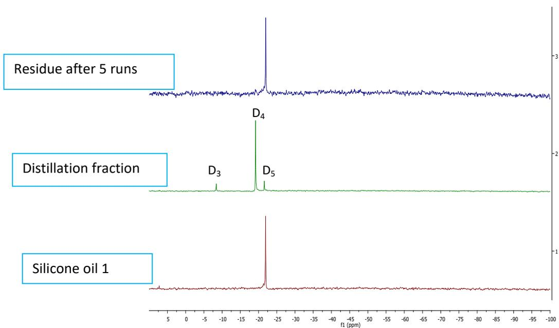
Figure S3: <sup>29</sup>Si-NMR of initial oil, distillation fraction and residue in *d*-chloroform
