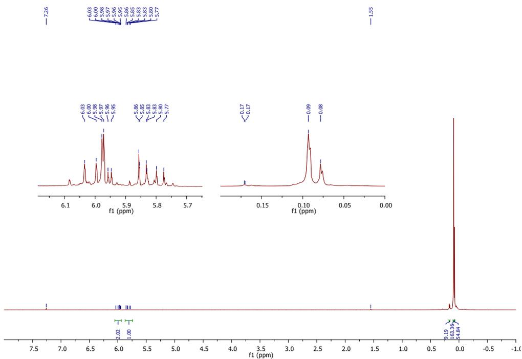
Figure S12:  $^1\text{H-NMR}$  spectrum of depolymerization products of silicone oil **7** ( $D_3$ ,  $D_4$ ,  $D_5$ ) (25°C,  $\text{CDCl}_3$ , 300 MHz)
