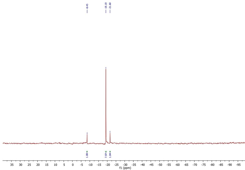
Figure S17:  $^{29}\text{Si}$ -NMR spectrum of depolymerization products of silicone oil **11** (25°C,  $\text{CDCl}_3$ , 59.6 MHz)
