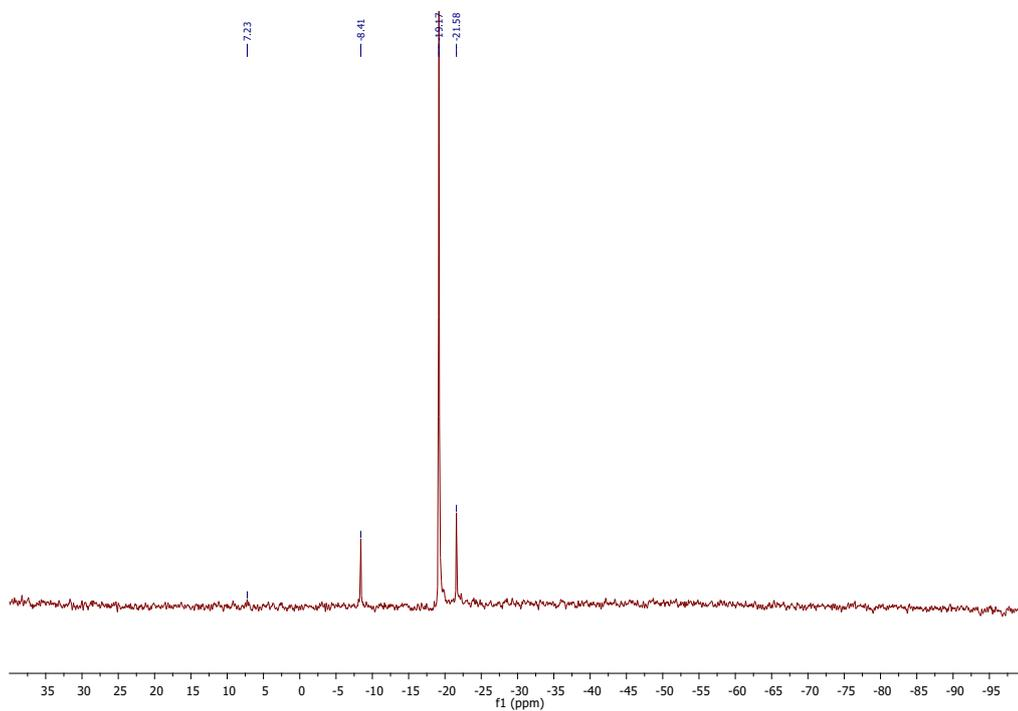
Figure S7:  $^{29}\text{Si}$ -NMR spectrum of depolymerization products of silicone oil **2** ( $D_3$ ,  $D_4$ ,  $D_5$ ) (25°C,  $\text{CDCl}_3$ , 59.6 MHz)
