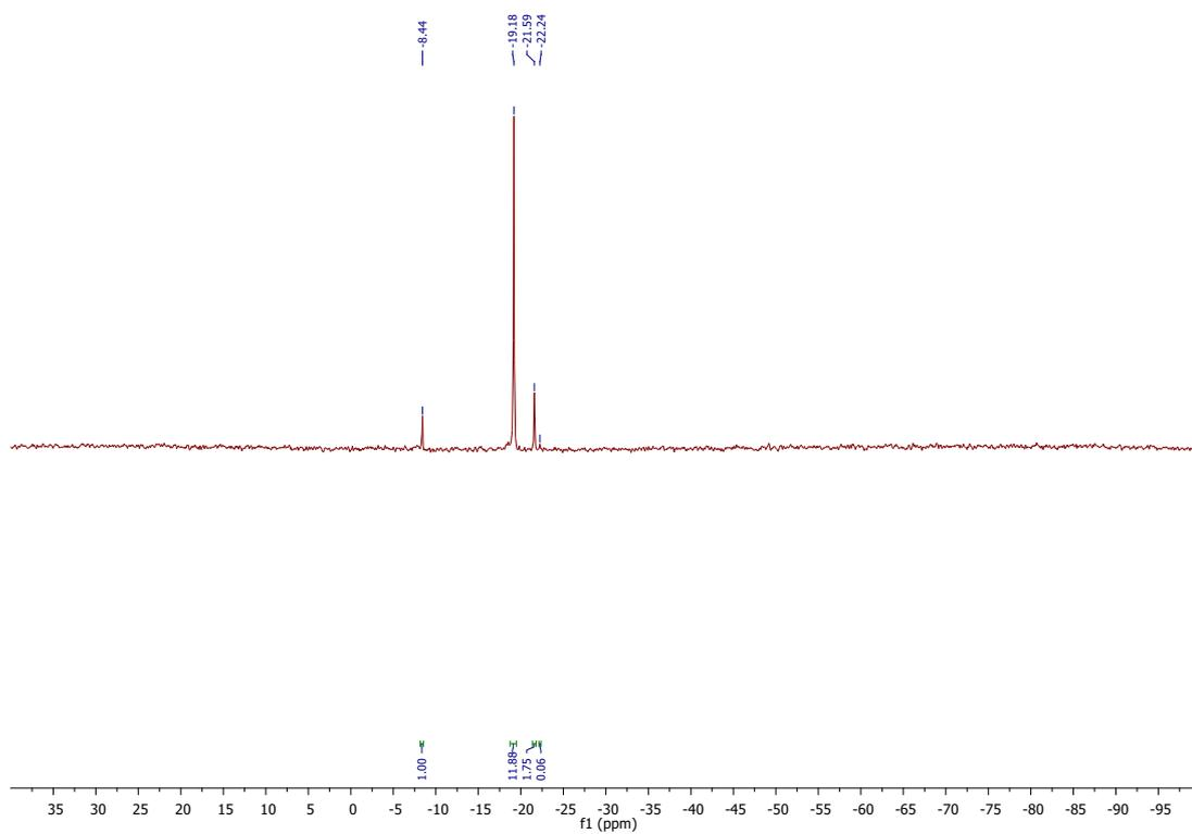
Figure S15:  $^{29}\text{Si}$ -NMR spectrum of depolymerization products of silicone oil **9 + 1** ( $D_3$ ,  $D_4$ ,  $D_5$ ) (25°C,  $\text{CDCl}_3$ , 59.6 MHz)
