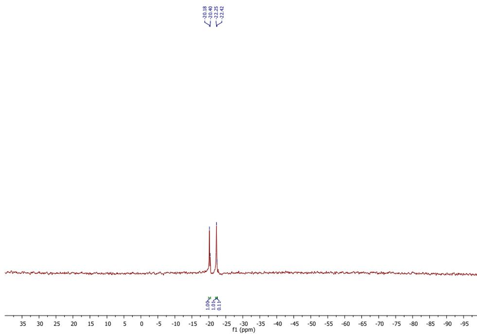
Figure S21:  $^{29}\text{Si}$ -NMR spectrum of depolymerization products of silicone oil **12** (25°C,  $d_6$ -acetone, 59.6 MHz)
