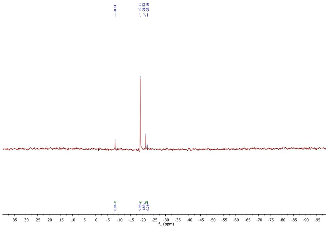
Figure S8:  $^{29}\text{Si}$ -NMR spectrum of depolymerization products of silicone gum **4 + 1** ( $D_3$ ,  $D_4$ ,  $D_5$ ) (25°C,  $\text{CDCl}_3$ , 59.6 MHz)
