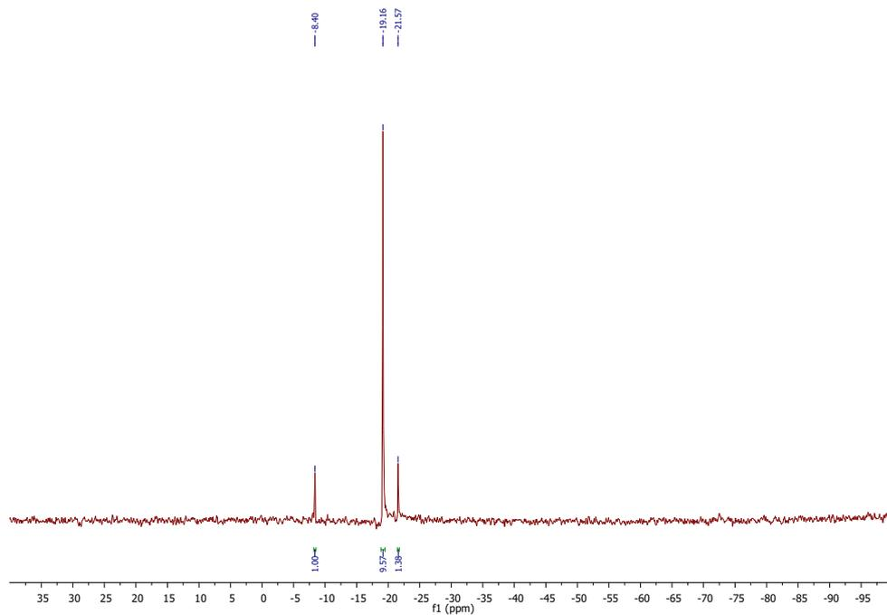
Figure S14:  $^{29}\text{Si}$ -NMR spectrum of depolymerization products of silicone oil **8 + 1** ( $D_3$ ,  $D_4$ ,  $D_5$ ) (25°C,  $\text{CDCl}_3$ , 59.6 MHz)
