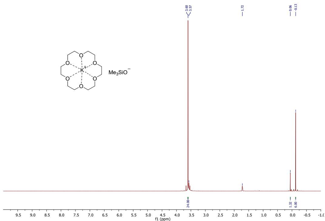
Figure S1a: <sup>1</sup>H-NMR of [KOSiMe<sub>3</sub>-18C6] complex in *d*<sub>8</sub>-THF (25°C, 300 MHz)
