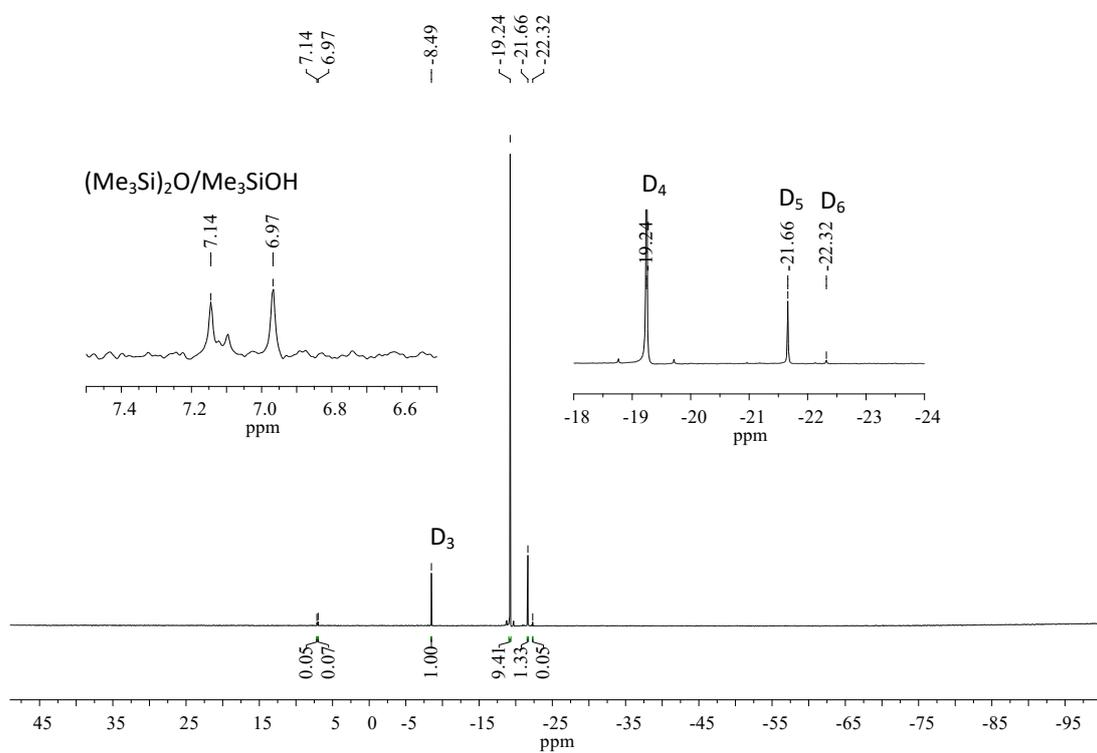
Figure S2: <sup>29</sup>Si-NMR of distillation fraction in *d*-chloroform (150 mg in 0.5 mL CDCl<sub>3</sub>, 25°C)
