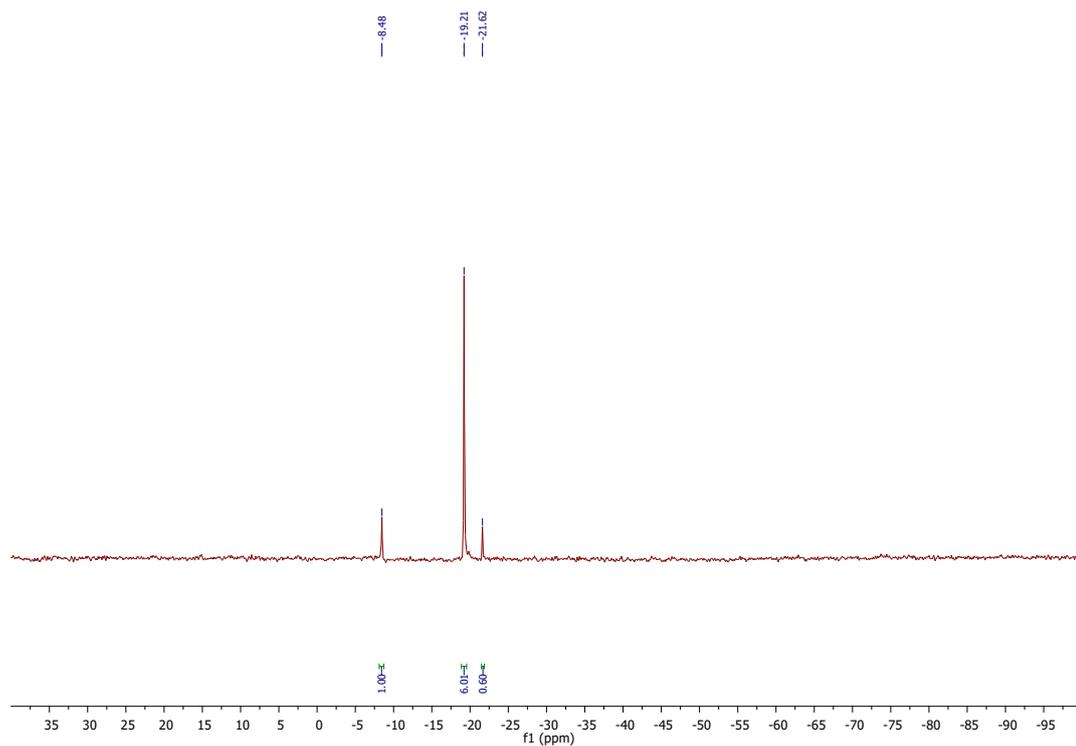
Figure S16:  $^{29}\text{Si}$ -NMR spectrum of depolymerization products of silicone oil **10 + 6 + 1** (25°C,  $\text{CDCl}_3$ , 59.6 MHz)
