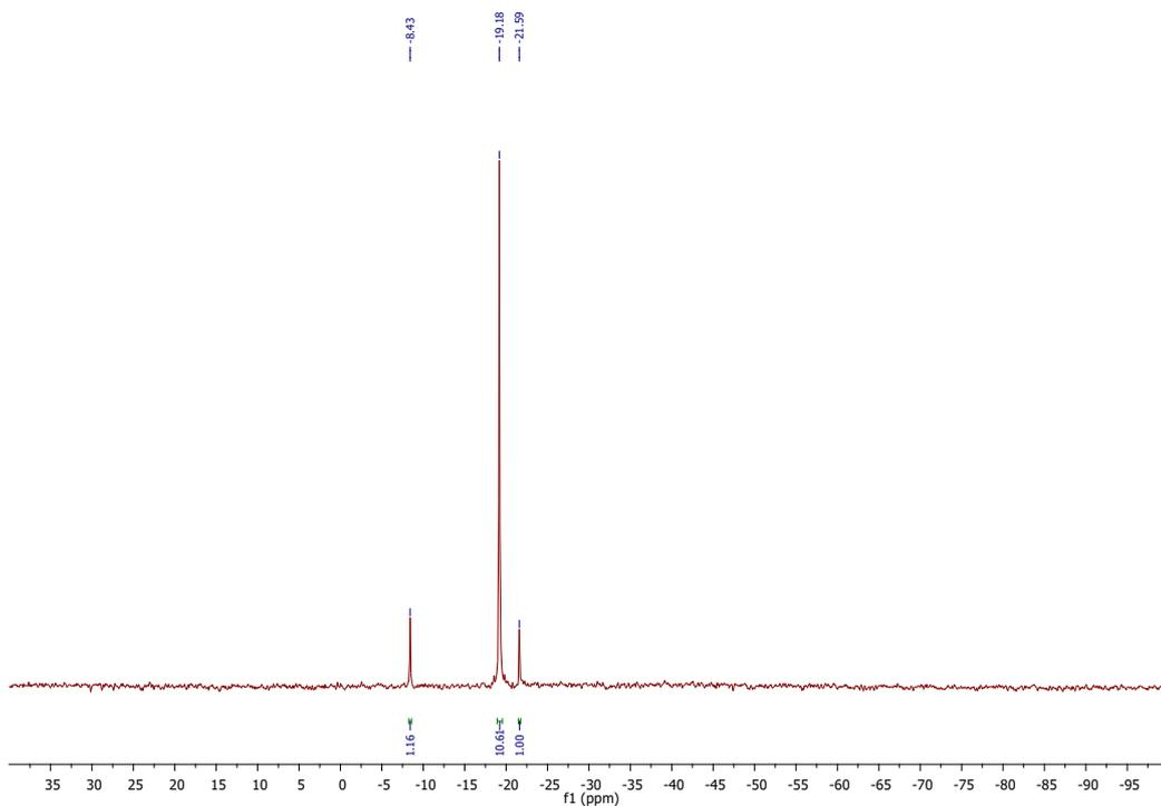
Figure S10:  $^{29}\text{Si}$ -NMR spectrum of depolymerization products of silicone oil **6** ( $D_3$ ,  $D_4$ ,  $D_5$ ) (25°C,  $\text{CDCl}_3$ , 59.6 MHz)
