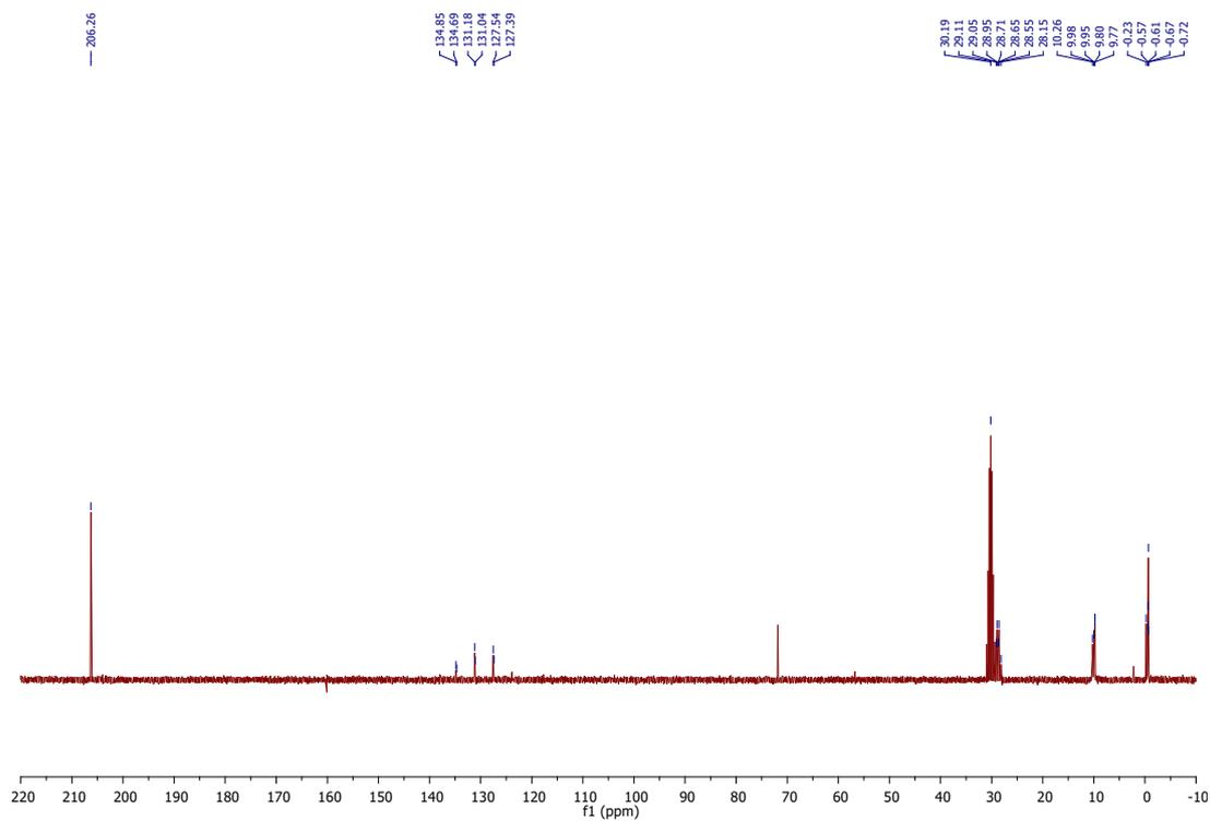
Figure S20:  $^{13}\text{C}$ -NMR spectrum of depolymerization products of silicone oil **12** (25°C,  $d_6$ -acetone, 75 MHz)
