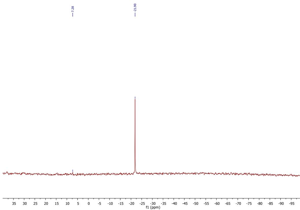
Figure S25:  $^{29}\text{Si}$ -NMR spectrum of lab-synthesized silicone oil (25°C,  $\text{CDCl}_3$ , 59.6 MHz)
