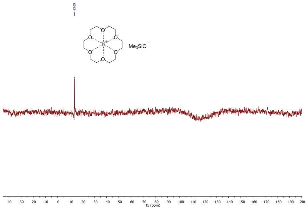
Figure S1c:  $^{29}\text{Si}$ -NMR of  $[\text{KOSiMe}_3\text{-18C6}]$  complex in  $d_8\text{-THF}$  (25°C, 59.6 MHz)
