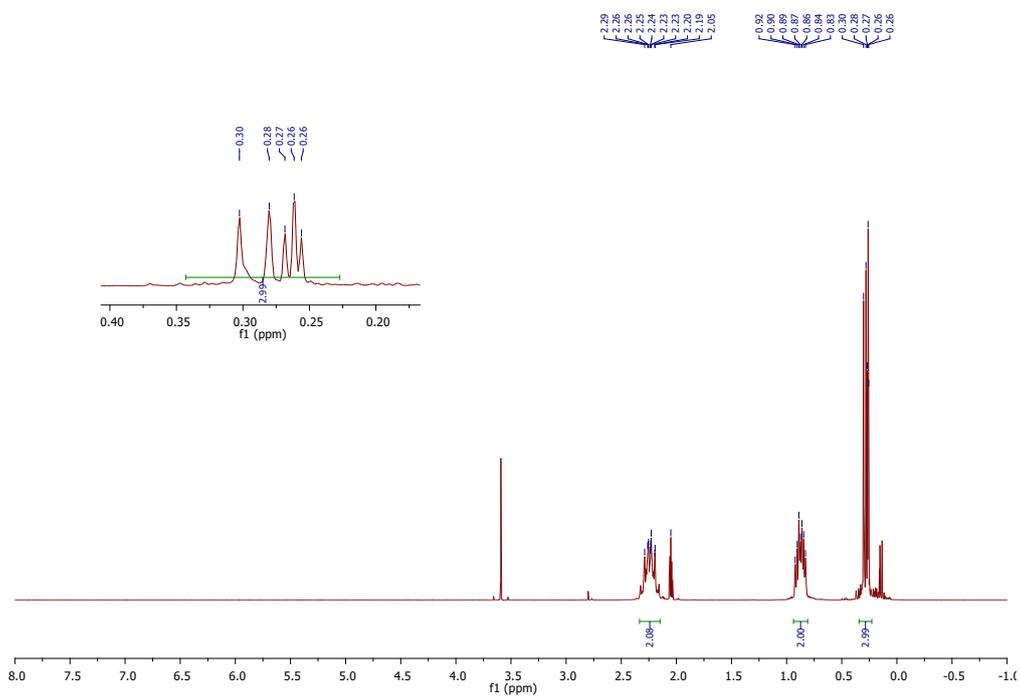
Figure S19:  $^1\text{H}$ -NMR spectrum of depolymerization products of silicone oil **12** (25°C,  $d_6$ -acetone, 300 MHz)
