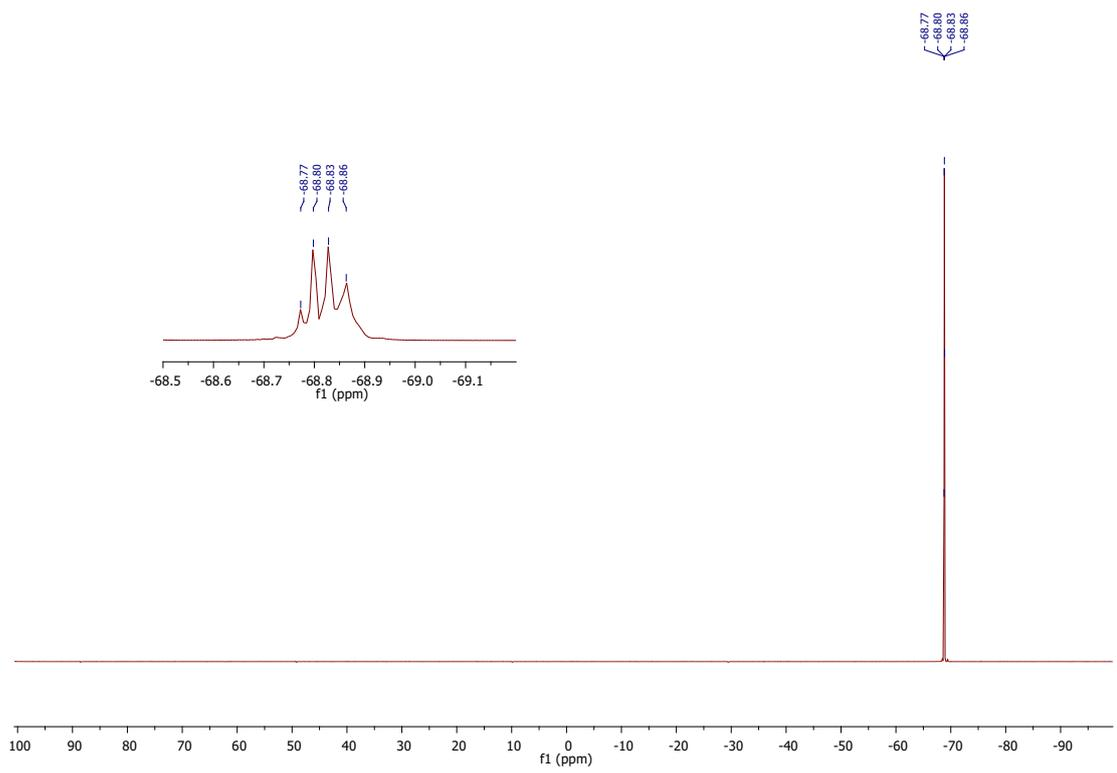
Figure S22:  $^{19}\text{F}$ -NMR spectrum of depolymerization products of silicone oil **12** (25°C,  $d_6$ -acetone, 284 MHz)
