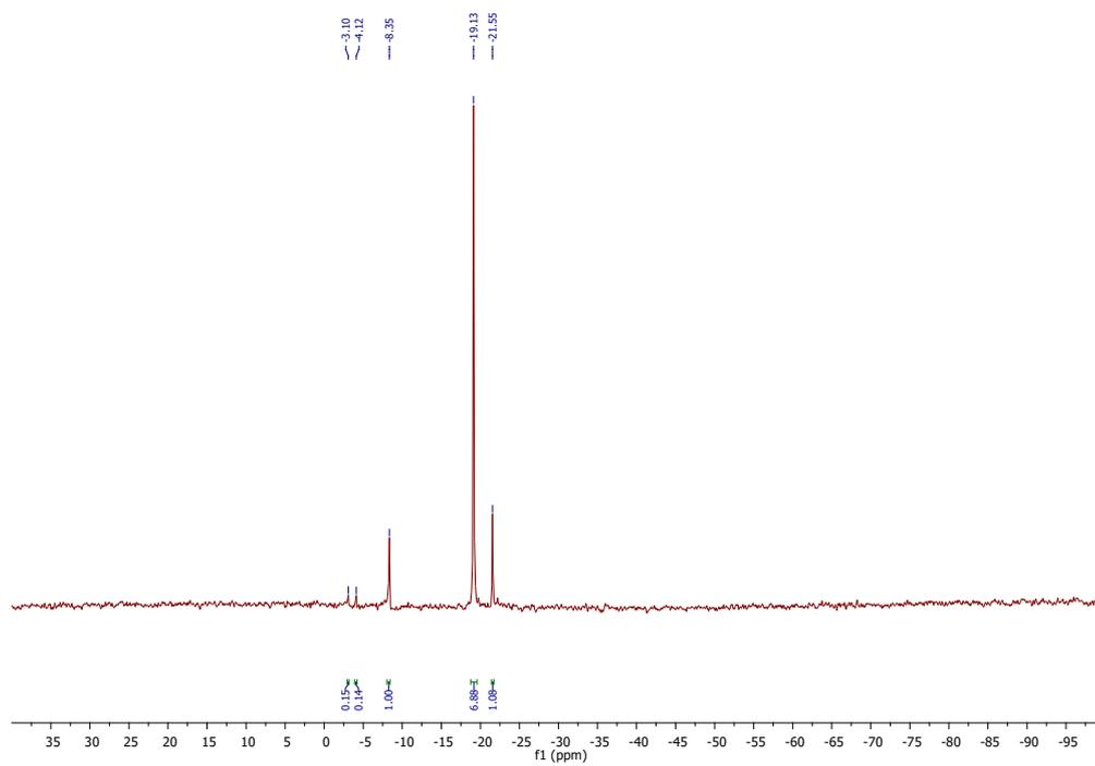
Figure S9:  $^{29}\text{Si}$ -NMR spectrum of depolymerization products of silicone oil **5** ( $D_3$ ,  $D_4$ ,  $D_5$ ) (25°C,  $\text{CDCl}_3$ , 59.6 MHz)
