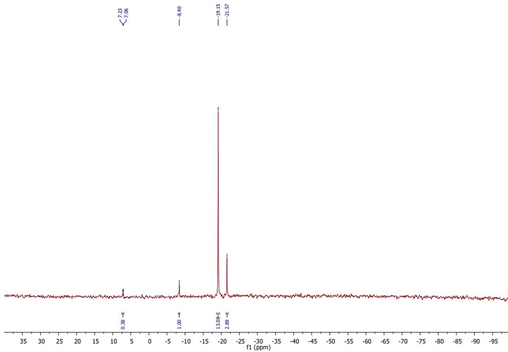
Figure S6:  $^{29}\text{Si}$ -NMR spectrum of depolymerization products of silicone oil **1** ( $D_3$ ,  $D_4$ ,  $D_5$ ) (25°C,  $\text{CDCl}_3$ , 59.6 MHz)
