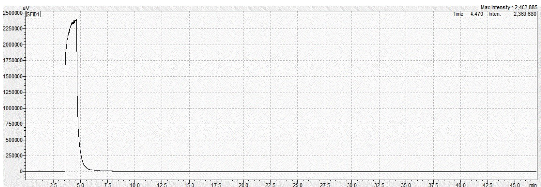
Fig. S12 The gas chromatography (GC) spectra of fresh ethylene glycol, ethylene glycol that was distilled after 6 recycles of glycolysis reaction and ethylene glycol, which was distilled after decolorization of sample 1. The characterization conditions: InertCap CHRAMIX, 30m×0.25mm, df = 2.5\mu\text{m} , nitrogen gas as a mobile phase at a column pressure of 5 psi. The injector and the FID temperatures were 275 °C. The column oven temperature procedure: 90 °C for 15min, 5 °C /min to 150 °C for 20 minutes.
