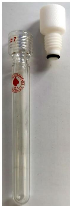
Figure S3: pressure tubes for investigations on mixing temperatures.
