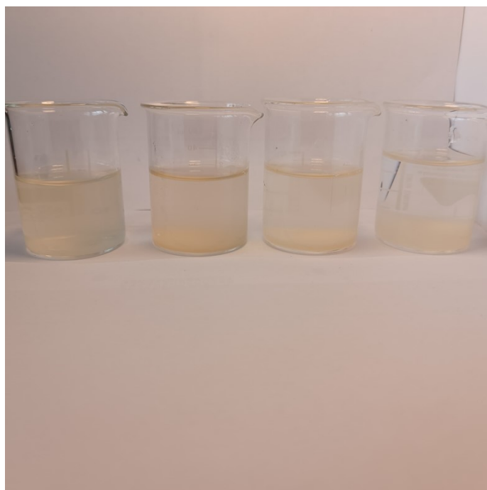
Figure S3. From left to right: the DS40, DS20, DS10 and chitosan samples after two days in a basic aqueous solution (pH = 12).
