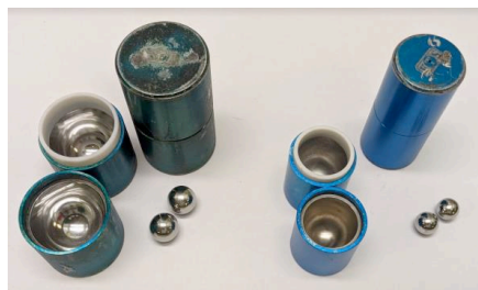
Formtech Scientific SMARTSNAP™ stainless steel grinding jars & Stainless steel balls.
