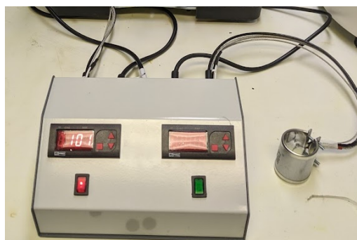
PID-controlled jar heater. - For more information click here
