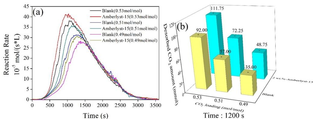
**Figure S3.** The CO<sub>2</sub> desorption performance with different initial CO<sub>2</sub> loading. (a) CO<sub>2</sub> desorption rate curves. (b) Total amount of CO<sub>2</sub> desorbed at 1200 s.
