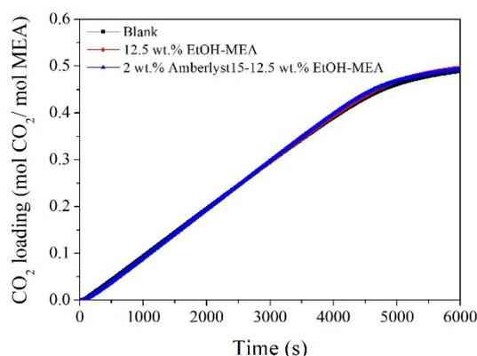
**Figure S9.** Influence of catalyst and ethanol solvent on CO<sub>2</sub> absorption performance.
