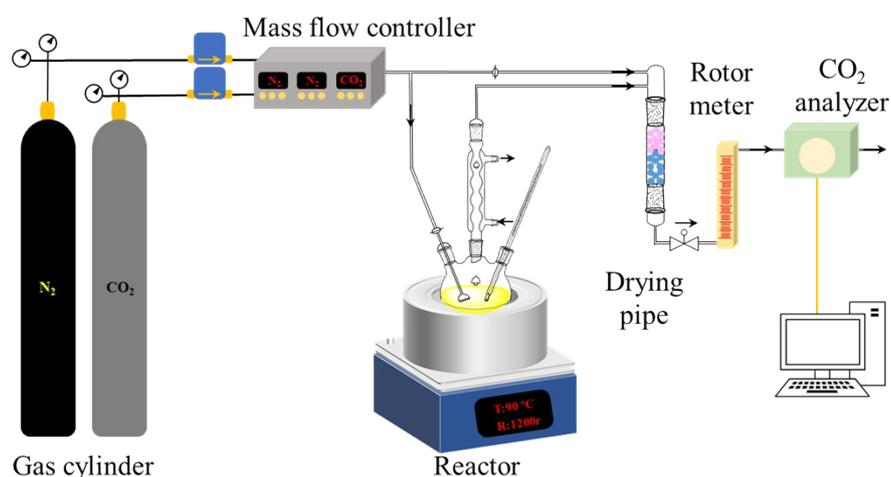
**Figure S1.** Schematic diagram of the experimental apparatus for CO<sub>2</sub> desorption and absorption.
