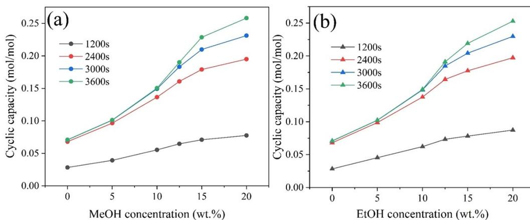
**Figure S7.** Comparison of cyclic capacity for the different alcohol-MEA systems at different regeneration time. (a) cyclic capacity of MeOH-MEA system. (b) cyclic capacity of EtOH-MEA system.
