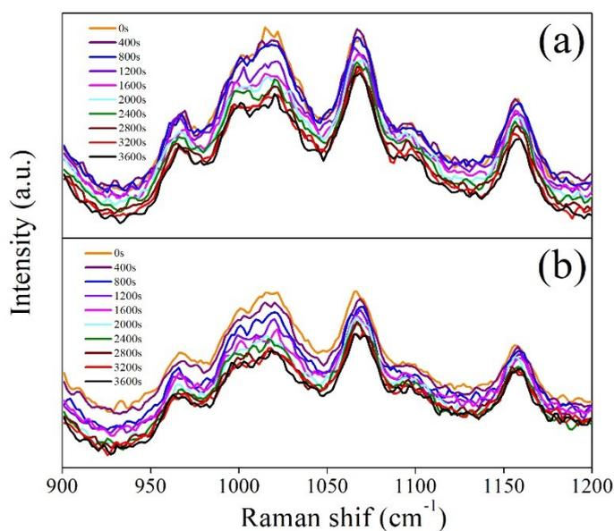
**Figure S4.** Raman spectra of MEA solution at various periods. (a) CO<sub>2</sub> desorption without catalyst. (b) CO<sub>2</sub> desorption with 2 wt.% Amberlyst-15.
