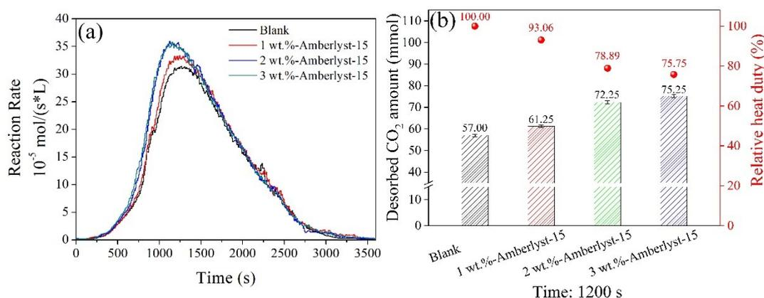
**Figure S5.** The CO<sub>2</sub> desorption performance with different catalyst/MEA solvent ratios. (a) CO<sub>2</sub> desorption rate curves. (b) Total amount of CO<sub>2</sub> desorbed and relative heat duty at 1200 s.
