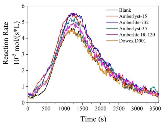
**Figure S2.** The CO<sub>2</sub> desorption rate curves with different catalysts at 80 °C.
