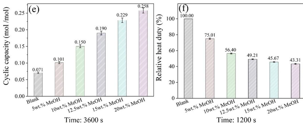
**Figure S6.** Effect of methanol concentration on CO<sub>2</sub> desorption performance at 90 °C.
