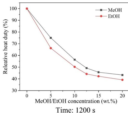
**Figure S8.** Comparison of relative heat duty for methanol and ethanol addition system at 1200 s.
