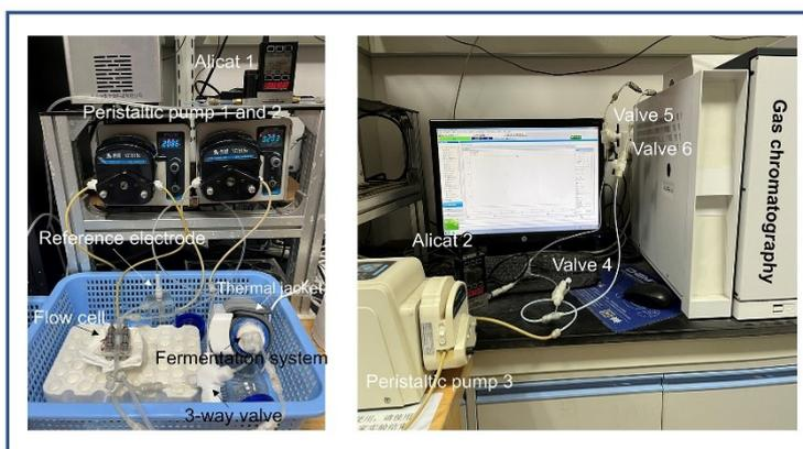
**Fig. S28** A photograph of the electro-bio reactor and the experimental setup. (The three-way valve replaced the valve 1, 2 and 3)
