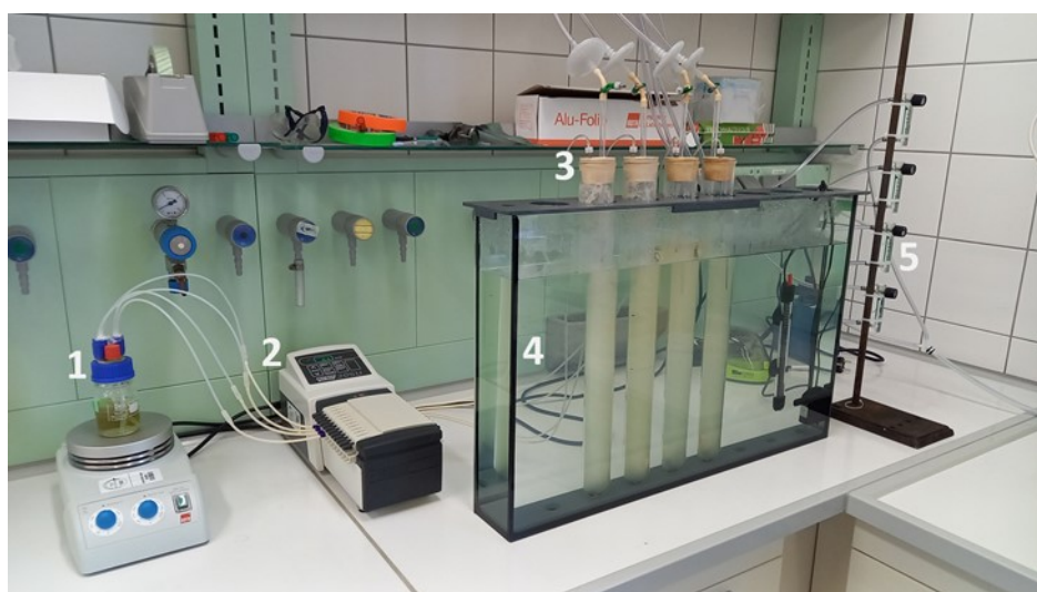
Figure S1. Experimental setup of bubble column bioreactors. 1: Substrate feedstock; 2: Pump with feeding line; 3: Bubble columns with 500 mL working volume; 4: Water bath with temperature regulation at 30 °C; 5: Gas supply line for 1 L min -1 sterile filtered air.
