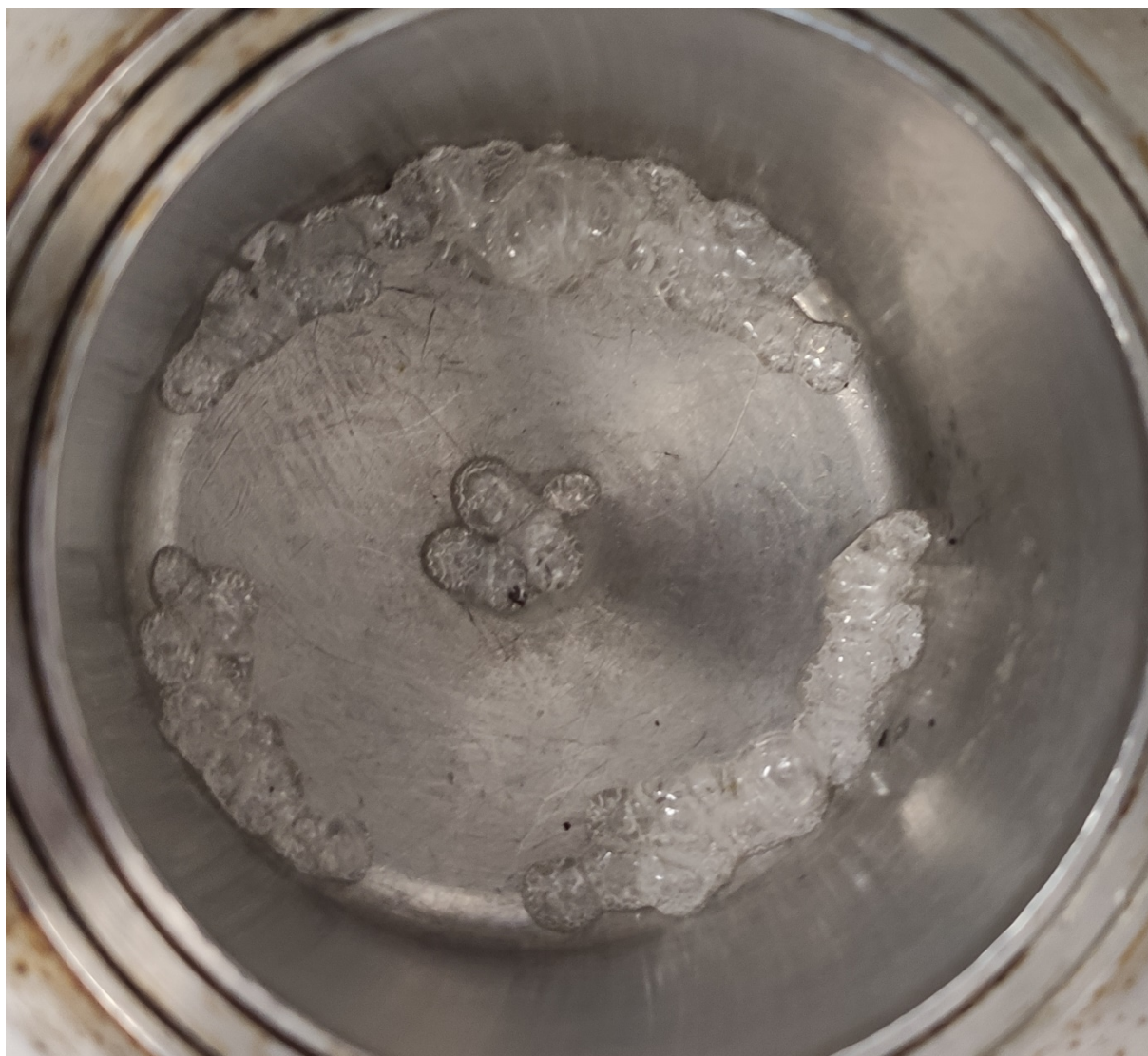
Photo S1. Open Batch reactor after a reaction in the absence of solvent (toluene): observation of “pop-corning” of pellets (after decompression of \text{CO}_2 ) and inhomogeneous reaction medium after carbonatation reaction.
