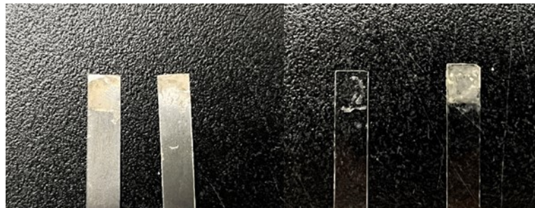
Figure S7 Photograph of cohesive failure on steel and interfacial failure on glass joined by 6-HTPB after testing at -40 °C.
