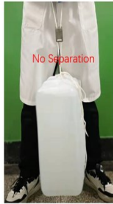
Figure S14 The view of steel plates (adhered by (6-HTPB) 20 -EG 1 adhesive, load of 25 kg) which had been stored for 100th day at 18 °C.
