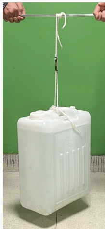
Figure S10 Macroscopic tests of (6\text{-HTPB})_{20}\text{-EG}_1 adhesive on steel at room temperature ( 17\text{ cm}^2 ; load of 50 kg). No separation or dislocation was observed.
