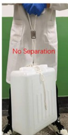
Figure S13 The view of steel plates (adhered by 6-HTPB adhesive, load of 25 kg) which had been stored for 6th day at 18 °C.
