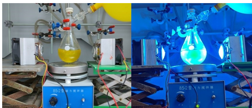
Supplementary figure 2 Photoreactor used in gram-scale synthesis (2 x 30W, 450 nm).
