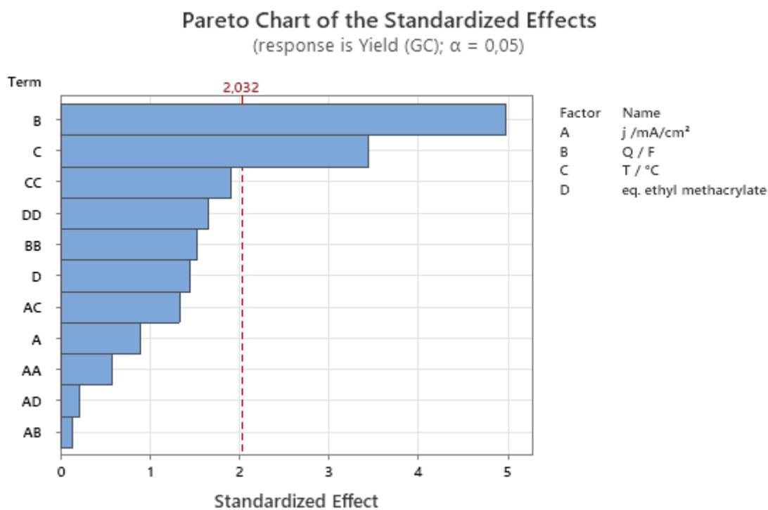
Figure S10: Pareto chart of the standardized effects for the first optimization of the biphasic synthesis of mefenpyr-diethyl (1) from **8b** via DoE.
