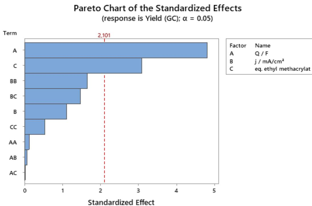
Figure S4: Pareto chart of the standardized effects for the first optimization of the synthesis of mefenpyr-diethyl (**1**) from **8a** via DoE.
