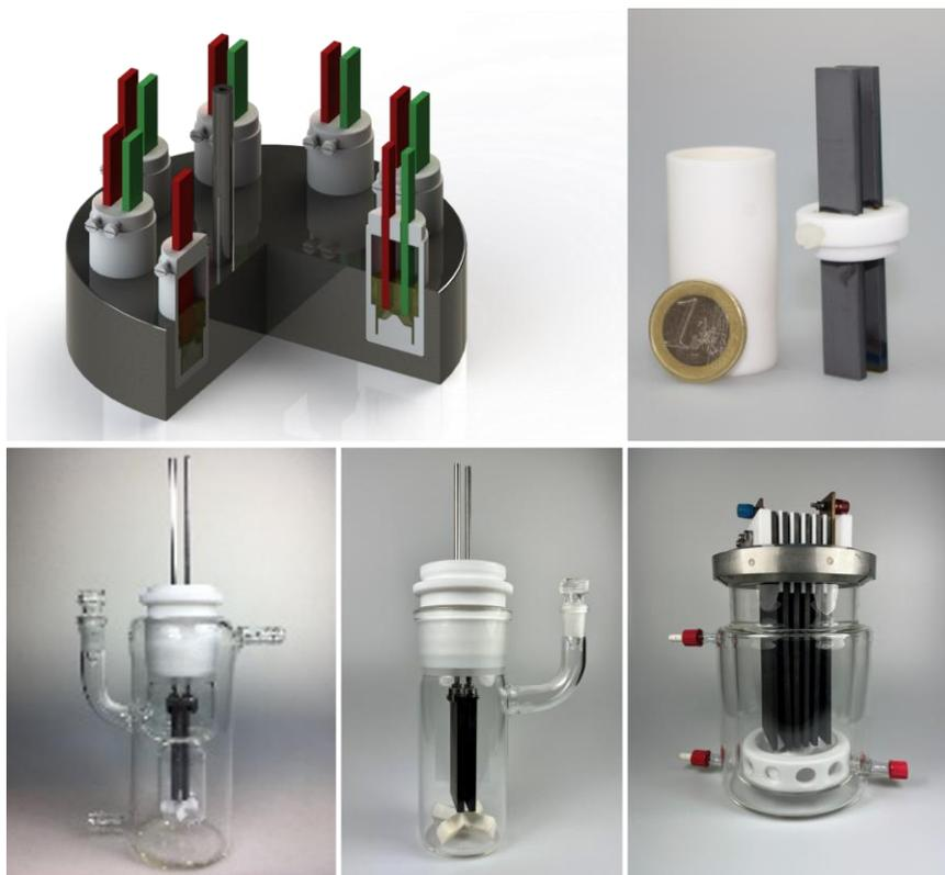
Figure S1: Top: schematic illustration of a screening block with undivided cells (left); undivided PTFE screening cell with BDD electrodes (right). Bottom: jacketed beaker-type cell, up to 50 mL reaction volume (left); beaker-type cell, up to 200 ml reaction volume (middle); jacketed beaker-type cell with 6 electrodes in a bipolar or stacked set-up, up to 1.5 L reaction volume (right).
