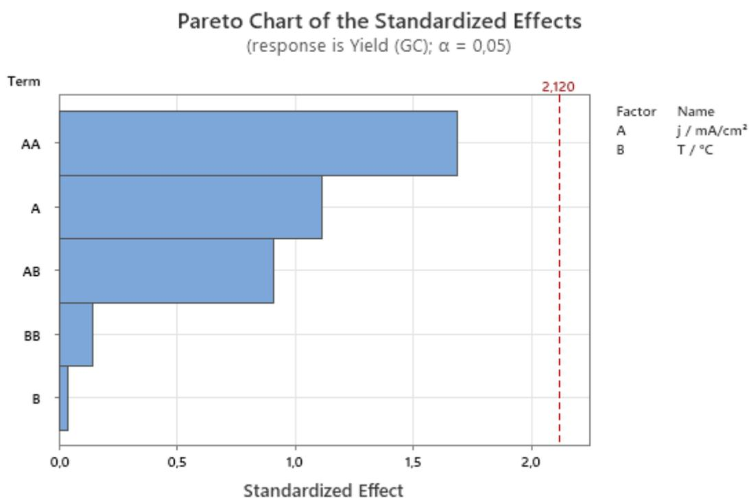
Figure S13: Pareto chart of the standardized effects for the second optimization of the biphasic synthesis of mefenpyr-diethyl (**1**) from **8b** via DoE.
