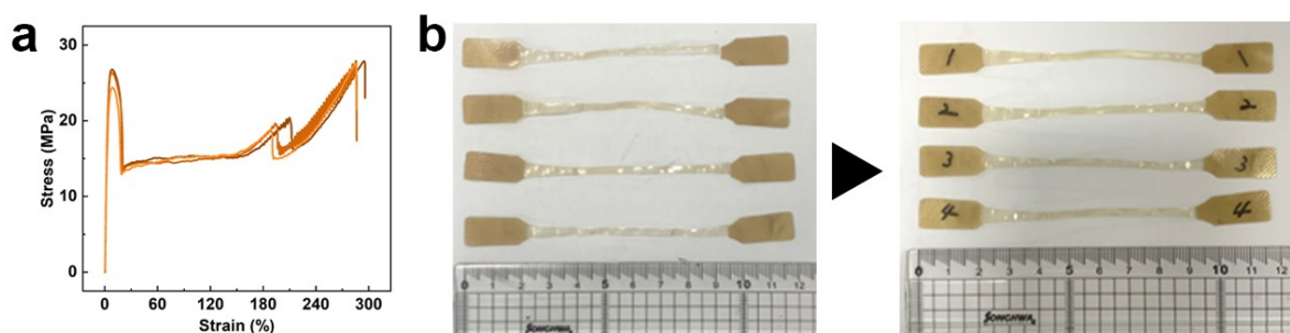
Figure S2. (a) Stress–strain curves for PPAT 70. (b) No change after elongation at break.
