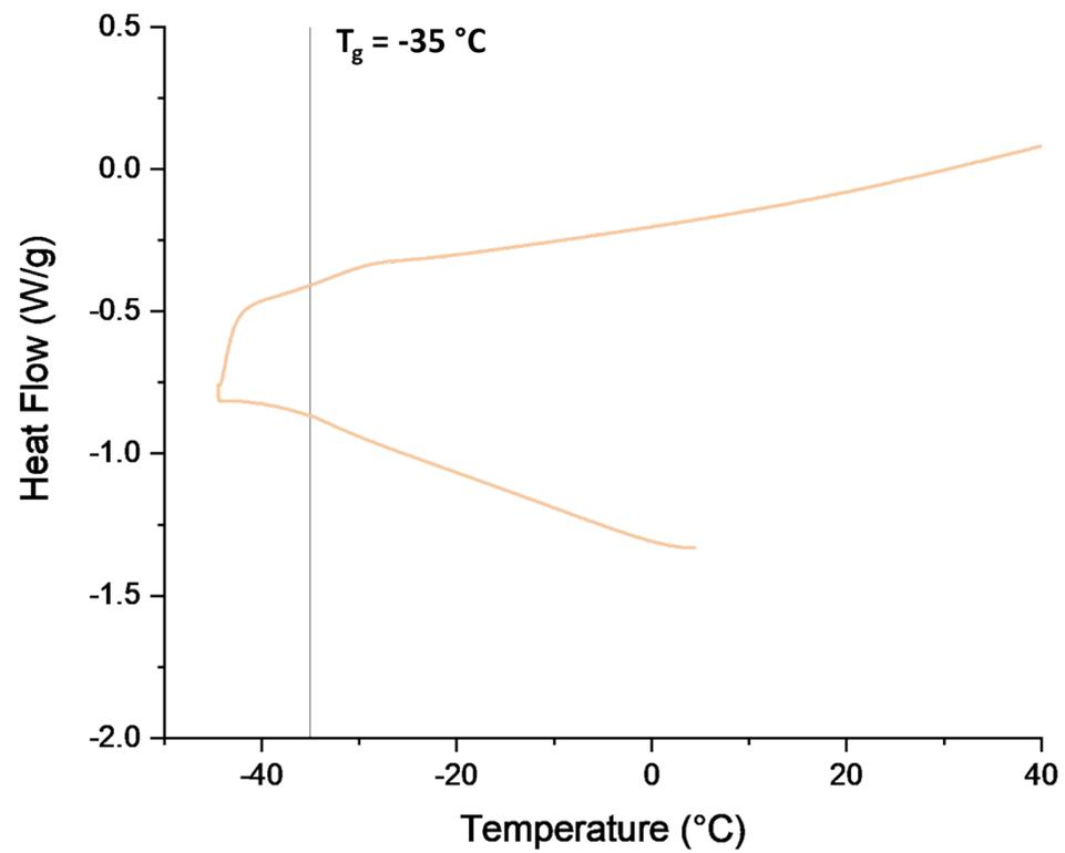
Figure S27. DSC curve of 1,2-epoxydecane:AGE = 50:50 polycarbonate (terpolymer).  $T_g$  determined from the heating branch (top).
