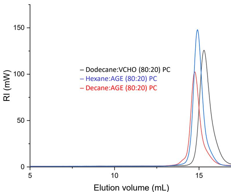
Figure S33. Examples of the monomodal GPC eluograms of the prepared terpolymers: 1,2-epoxydodecane:VCHO (80:20) terpolymer in black; 1,2-epoxyhexane:AGE (80:20) terpolymer in blue; 1,2-epoxydecane:AGE (80:20) terpolymer in red.
