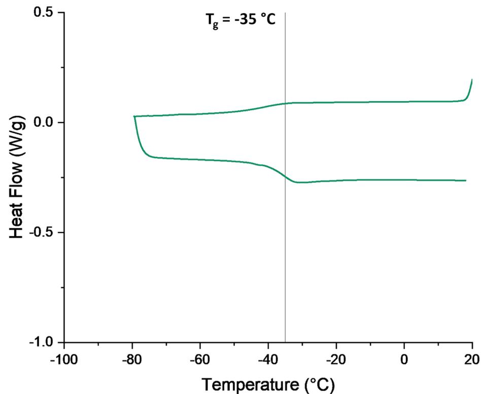
Figure S31. DSC curve of AGE polycarbonate (copolymer) prepared on large scale.  $T_g$  determined from the heating branch (bottom).
