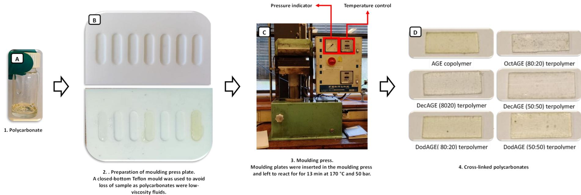
Figure S35. Cross-linking in a moulding press: (A) liquid polycarbonates before cross-linking; (B) a closed-bottom Teflon moulding plate to avoid polymers loss (the polycarbonates before cross-linking are low-viscosity fluids); (C) moulding press set-up; and (D) final cross-linked polycarbonates (solid).
