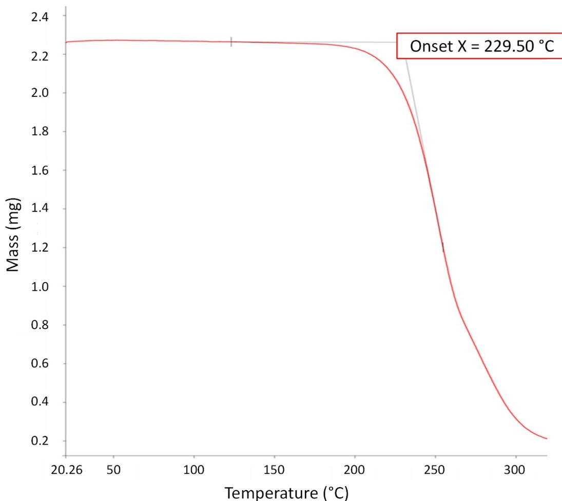
Figure S34. TGA of 1,2-epoxydecane:AGE = 80:20 polycarbonate (terpolymer). The temperature of the onset of the degradation was calculated as the intersection of the two tangents to the curve.
