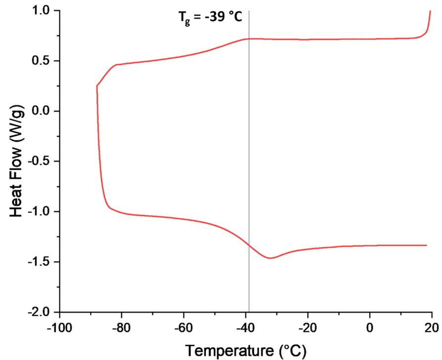
Figure S17. DSC curve of 1,2-epoxydecane polycarbonate (copolymer).  $T_g$  determined from the heating branch (bottom).
