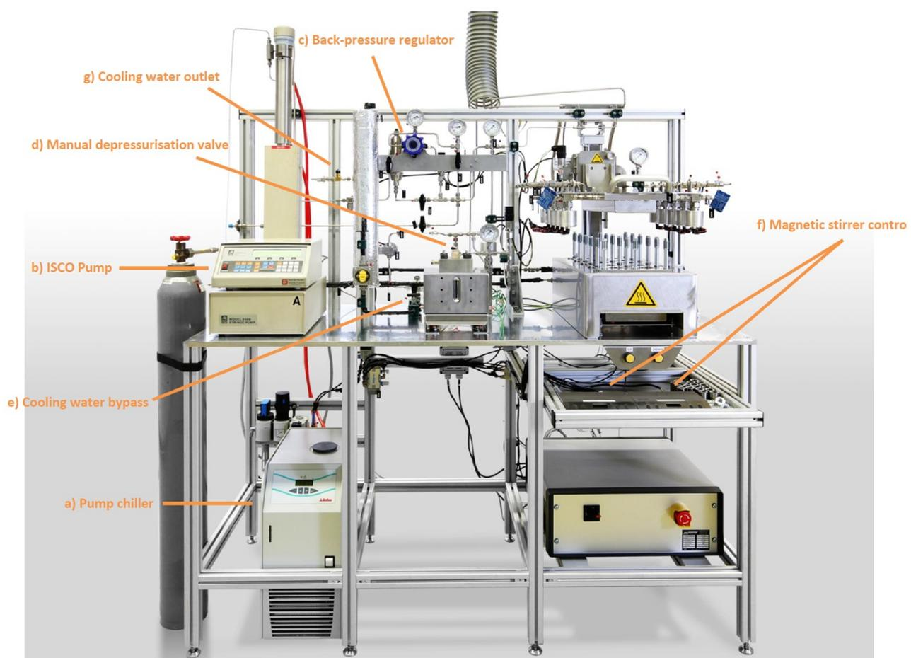
Figure S2. High-throughput unit used to perform the reactions with CO<sub>2</sub>.
