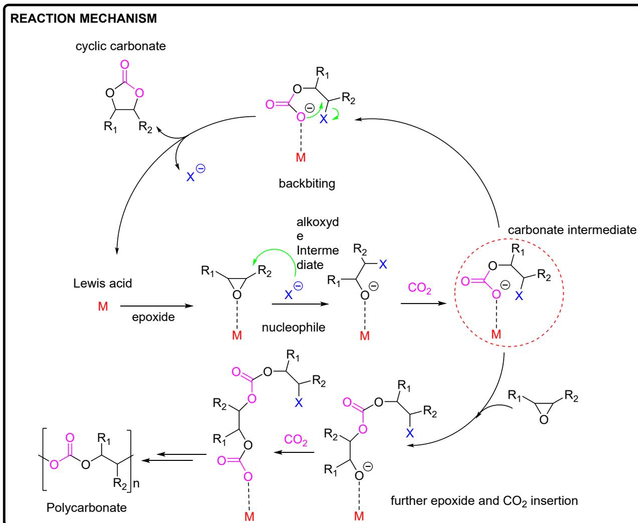
Figure S1. Proposed reaction mechanism for the coupling reaction between carbon dioxide and epoxides.
