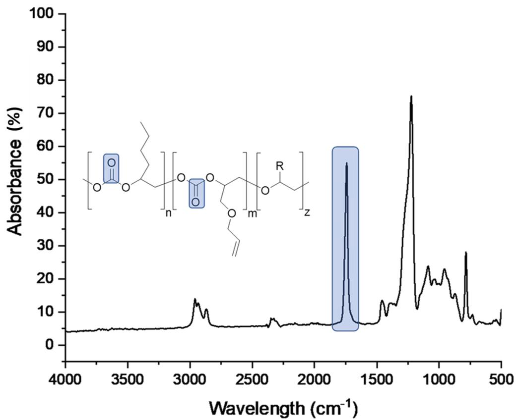
Figure S10. FT-IR spectrum of the crude mixture after the terpolymerisation of 1,2-epoxyhexane and AGE (80:20) with CO<sub>2</sub> (top) and of the purified polycarbonate (bottom).
