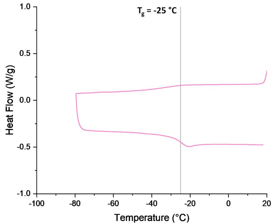
Figure S21. DSC curve of 1,2-epoxyhexane:AGE = 50:50 polycarbonate (terpolymer).  $T_g$  determined from the heating branch (bottom).
