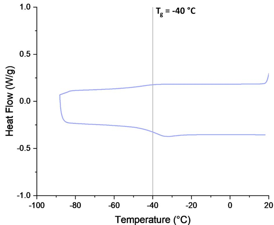
Figure S30. DSC curve of 1,2-epoxydodecane:AGE = 50:50 polycarbonate (terpolymer).  $T_g$  determined from the heating branch (bottom).
