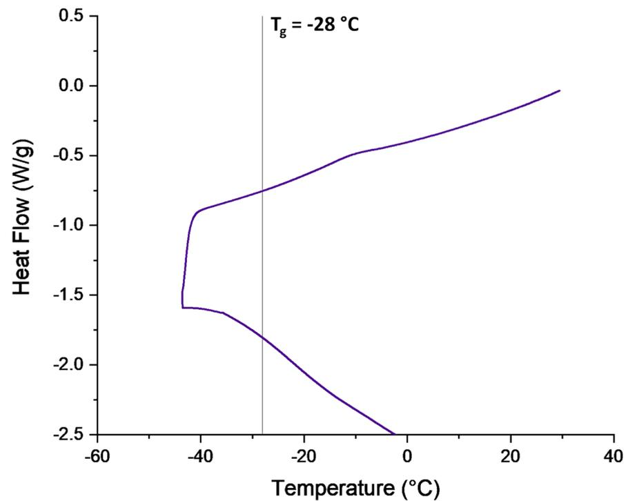
Figure S16. DSC curve of 1,2-epoxyoctane polycarbonate (copolymer).  $T_g$  determined from the heating branch (top).
