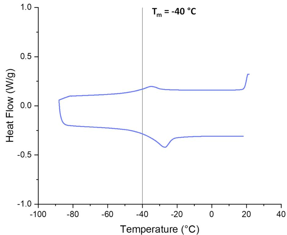
Figure S29. DSC curve of 1,2-epoxydodecane:AGE = 80:20 polycarbonate (terpolymer).  $T_m$  determined from the heating branch (bottom).
