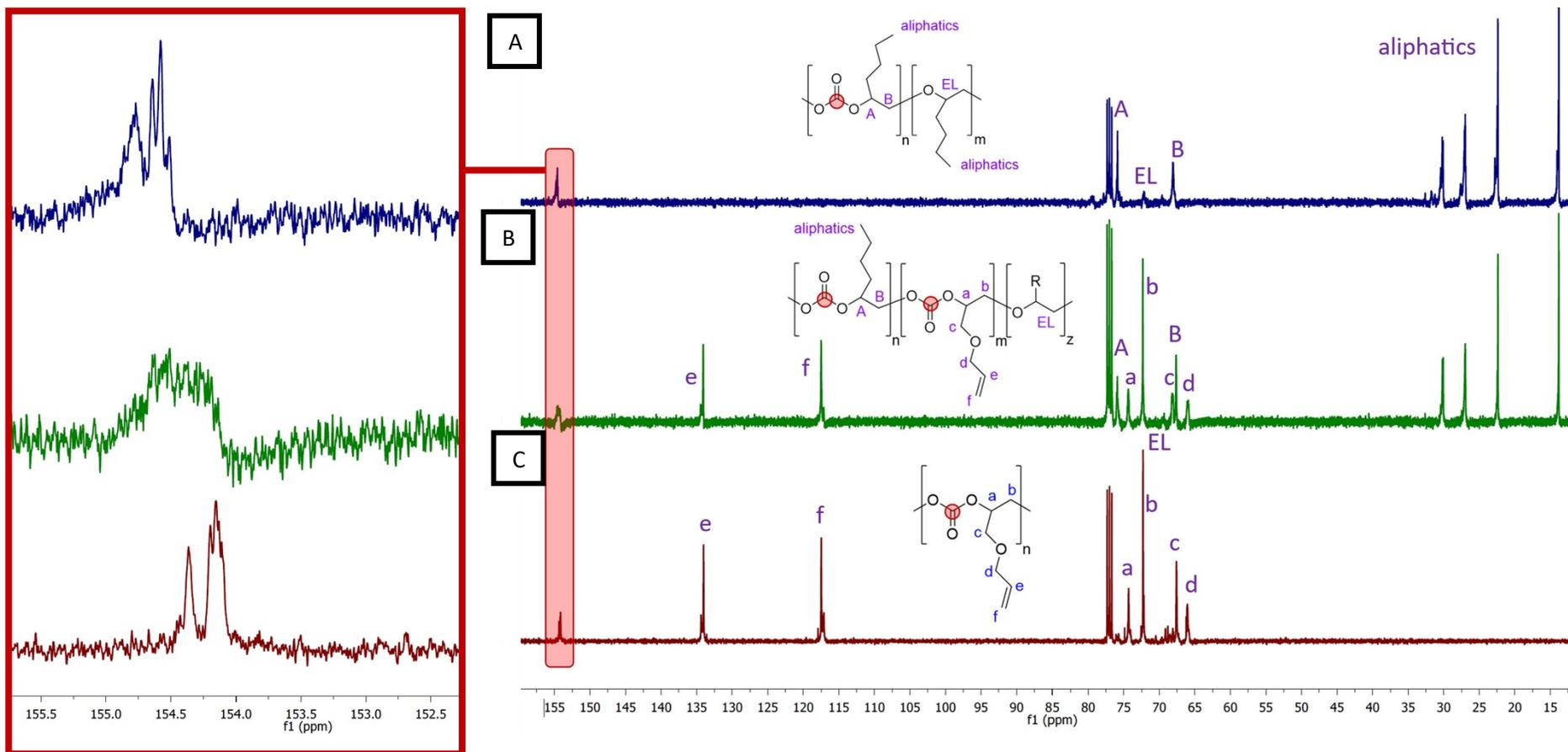
Figure S13.  $^{13}\text{C}$  NMR spectra of: (A) polycarbonate copolymer of 1,2-epoxyhexane, in blue; (B) polycarbonate terpolymer of 1,2-epoxyhexane:AGE = 50:50, in green; and (C) polycarbonate copolymer of AGE, in red. The region of the signals of PC carbonyls is highlighted in burgundy red. On the left: zoom-in of the carbonate signals of the three samples; no preferential polymerisation regiochemistry was observed in the terpolymerisation (random terpolymer, in green).
