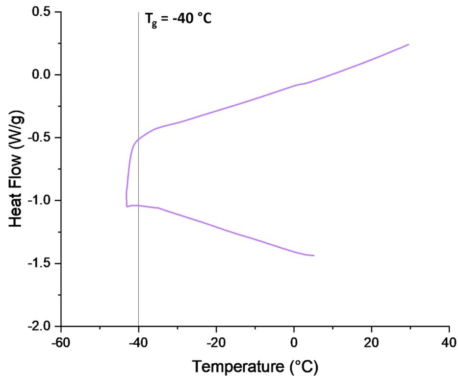
Figure S24. DSC curve of 1,2-epoxyoctane:AGE = 50:50 polycarbonate (terpolymer).  $T_g$  determined from the heating branch (top).
