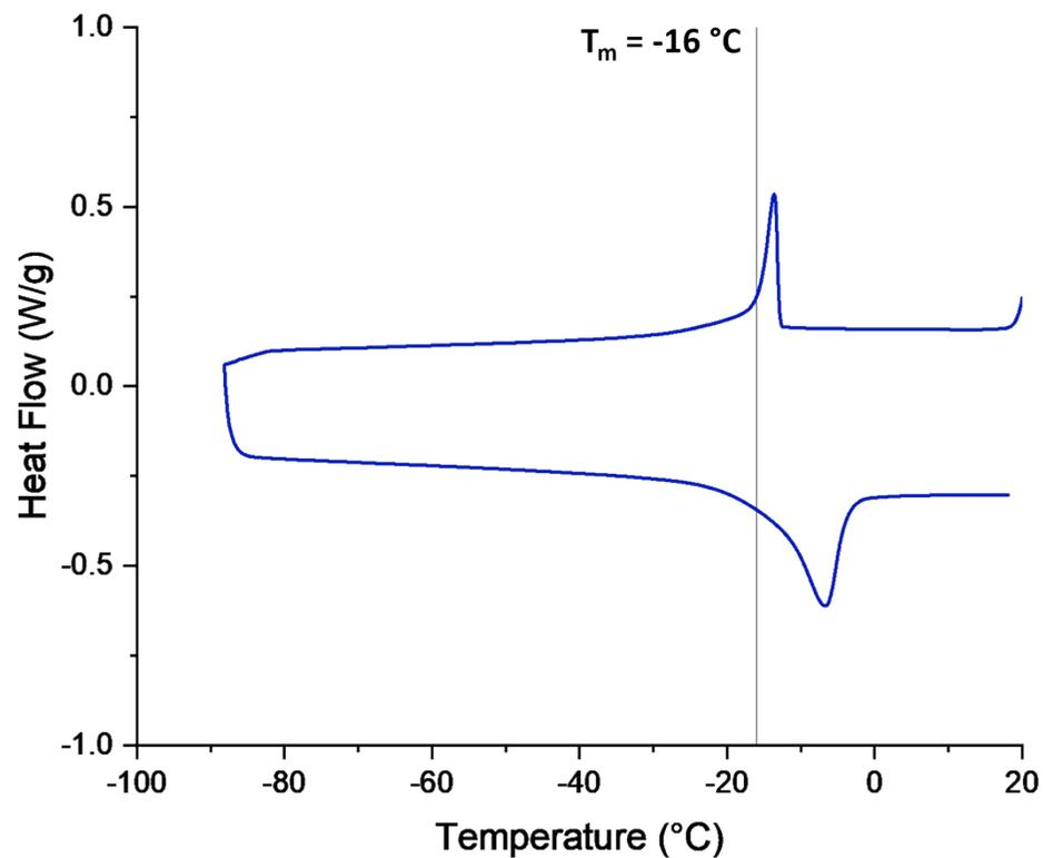
Figure S18. DSC curve of 1,2-epoxydodecane polycarbonate (copolymer).  $T_m$  determined from the heating branch (bottom).
