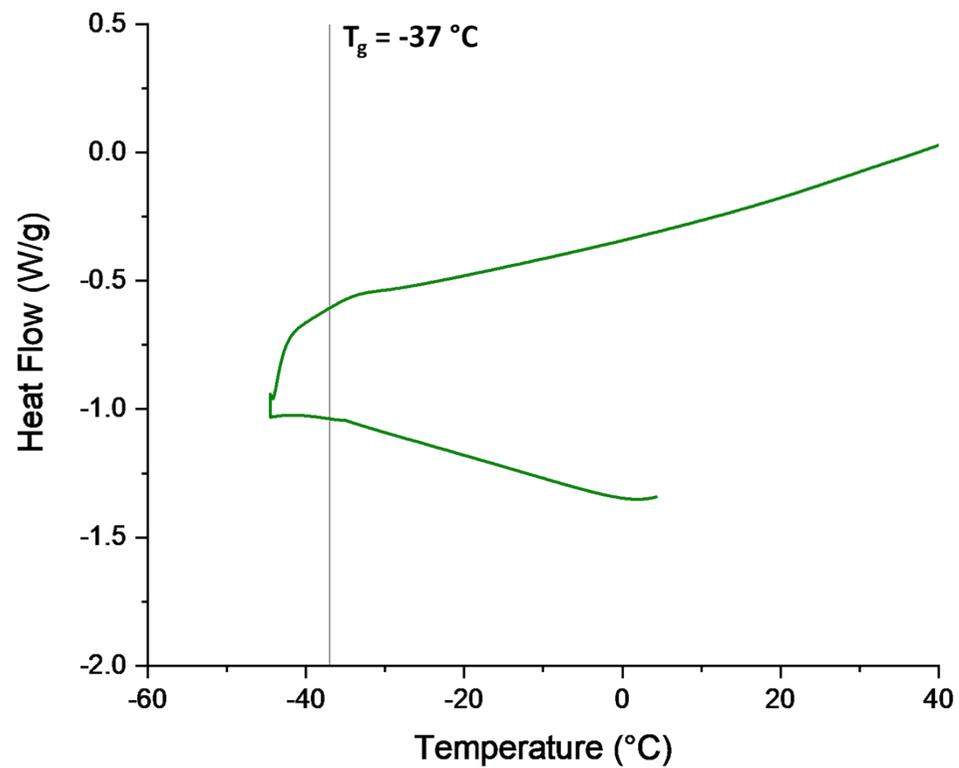
Figure S14. DSC curve of AGE polycarbonate (copolymer).
