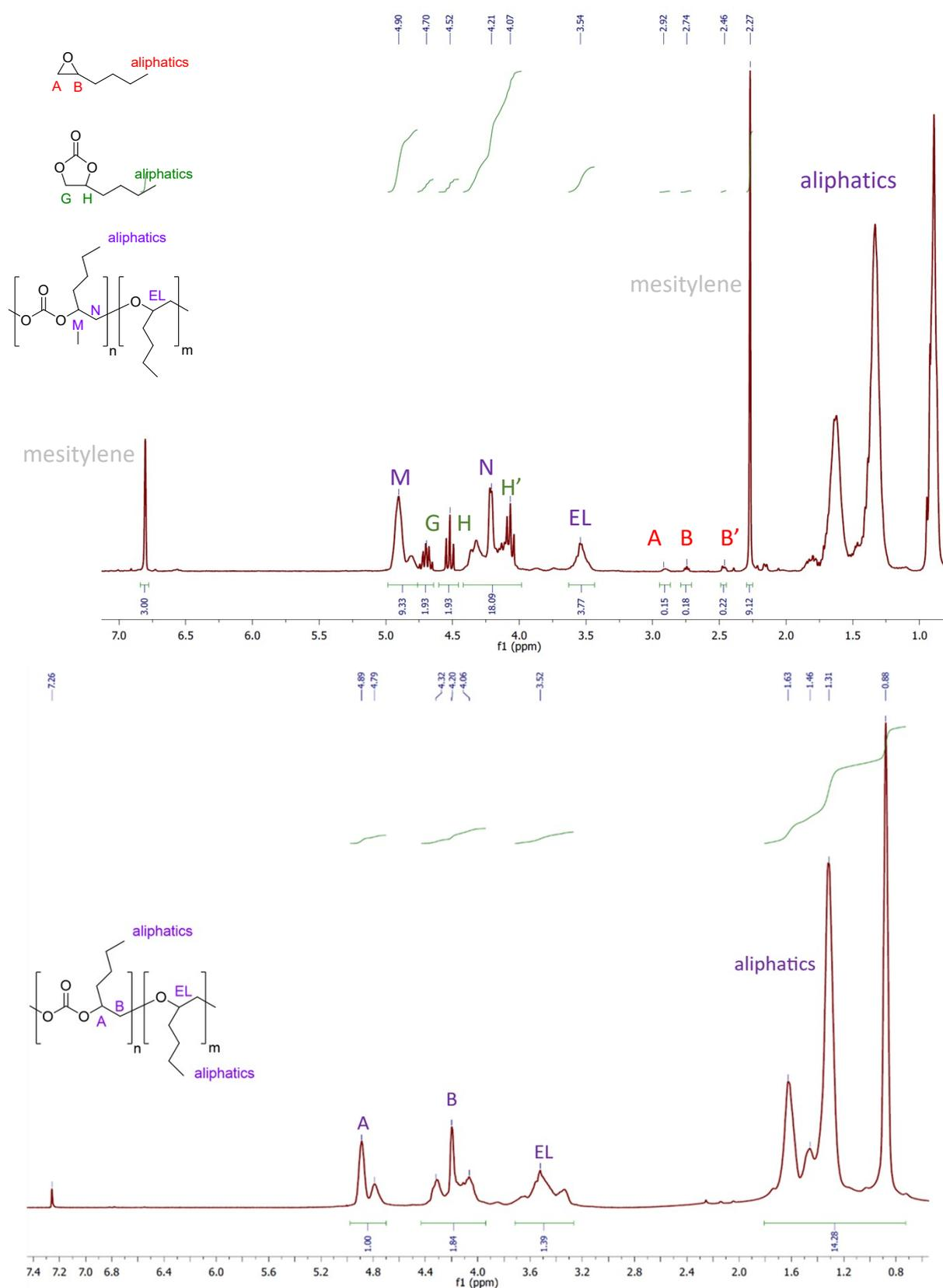
Figure S3.  $^1\text{H}$  NMR spectrum of the crude mixture after the copolymerisation of 1,2-epoxyhexane with  $\text{CO}_2$  (top) and of the purified polycarbonate (bottom).
