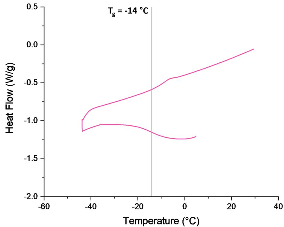
Figure S20. DSC curve of 1,2-epoxyhexane:AGE = 80:20 polycarbonate (terpolymer).  $T_g$  determined from the heating branch (top).
