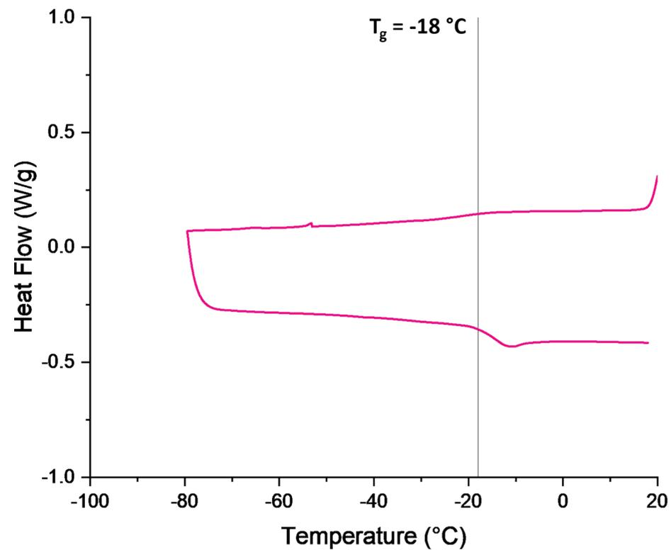
Figure S19. DSC curve of 1,2-epoxyhexane:AGE = 95:5 polycarbonate (terpolymer).  $T_g$  determined from the heating branch (bottom).
