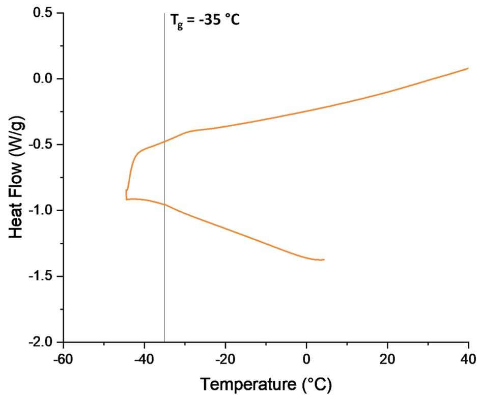
Figure S26. DSC curve of 1,2-epoxydecane:AGE = 80:20 polycarbonate (terpolymer).  $T_g$  determined from the heating branch (top).
