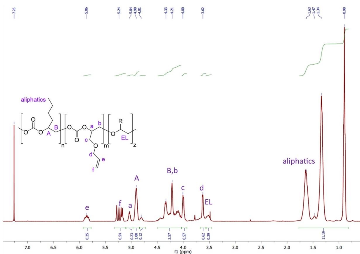
Figure S9.  $^1\text{H}$  NMR spectrum of the crude mixture after the terpolymerisation of 1,2-epoxyhexane and AGE (80:20) with  $\text{CO}_2$  (top) and of the purified polycarbonate (bottom).
