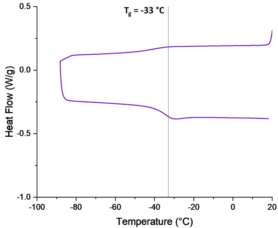
Figure S22. DSC curve of 1,2-epoxyoctane:AGE = 95:5 polycarbonate (terpolymer).  $T_g$  determined from the heating branch (bottom).
