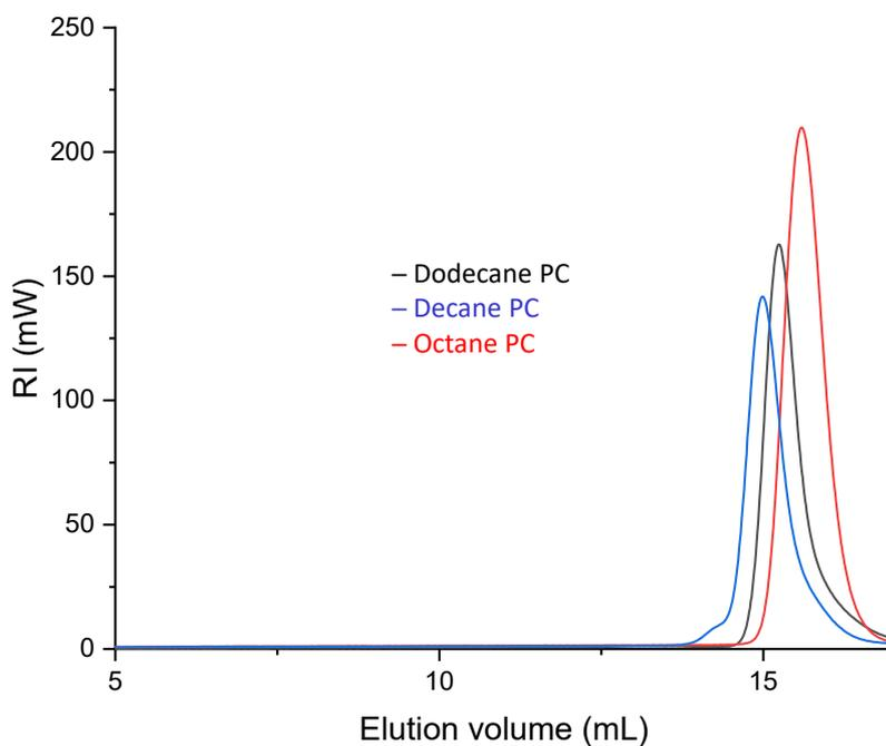
Figure S32. Examples of the monomodal GPC eluograms of the prepared copolymers: 1,2-epoxydodecane-based copolymer in black; 1,2-epoxydecane-based copolymer in blue; 1,2-epoxyoctane-based copolymer in red.
