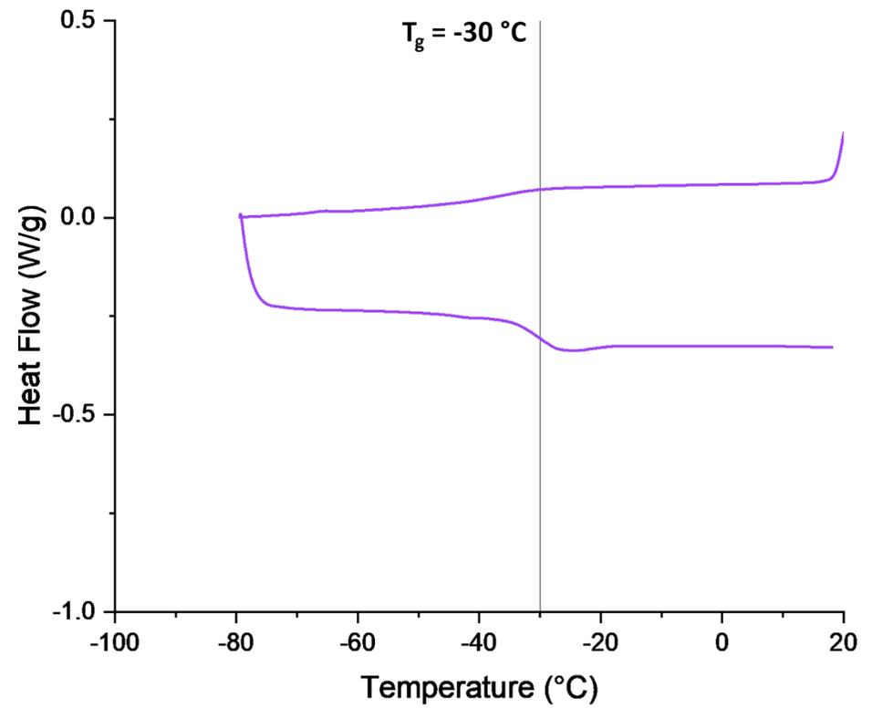
Figure S23. DSC curve of 1,2-epoxyoctane:AGE = 80:20 polycarbonate (terpolymer).  $T_g$  determined from the heating branch (bottom).
