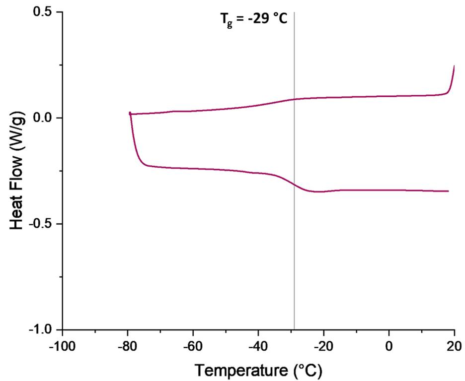
Figure S15. DSC curve of 1,2-epoxyhexane polycarbonate (copolymer).
