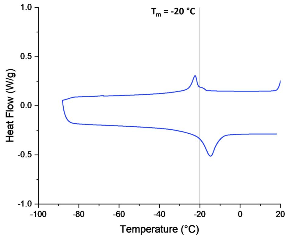
Figure S28. DSC curve of 1,2-epoxydodecane:AGE = 95:5 polycarbonate (terpolymer).  $T_m$  determined from the heating branch (bottom).
