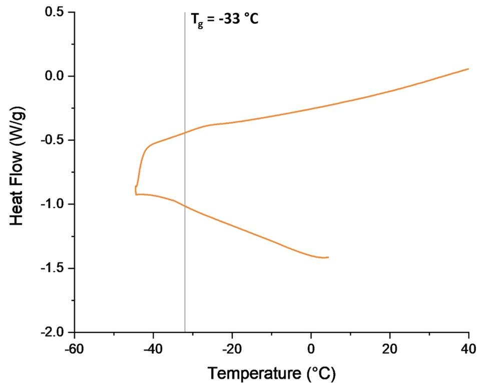
Figure S25. DSC curve of 1,2-epoxydecane:AGE = 95:5 polycarbonate (terpolymer).  $T_g$  determined from the heating branch (top).
