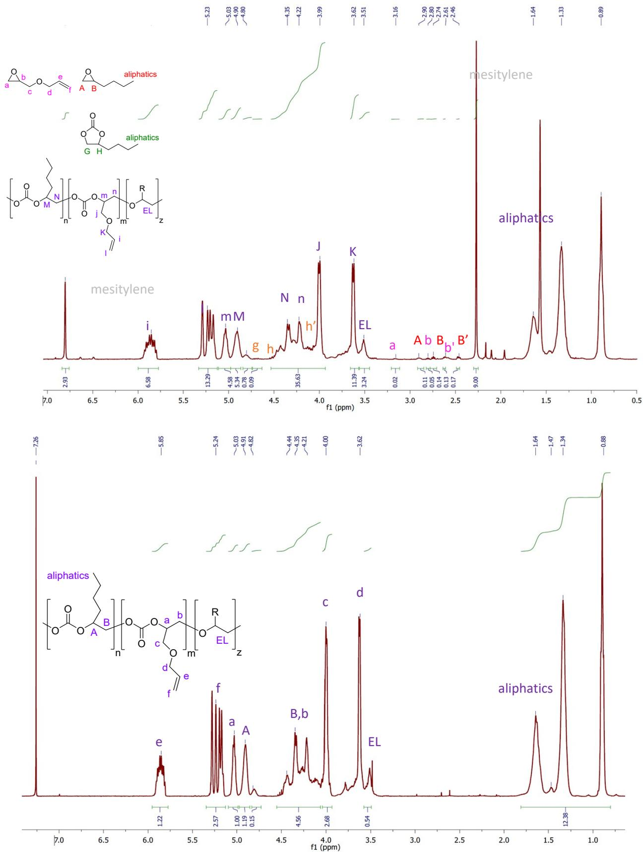
Figure S11.  $^1\text{H}$  NMR spectrum of the crude mixture after the terpolymerisation of 1,2-epoxyhexane and AGE (50:50) with  $\text{CO}_2$  (top) and of the purified polycarbonate (bottom).
