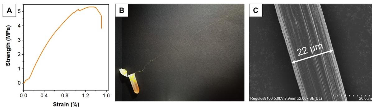
**Figure S27.** Mechanical properties of P1a2aCS<sub>2</sub>. (A) The stretch curve of P1a2aCS<sub>2</sub> tested by electronic universal testing machine. (B) The continuous fiber of P1a2aCS<sub>2</sub> prepared through solution processing and (C) the scanning electron microscope image of this fiber.
