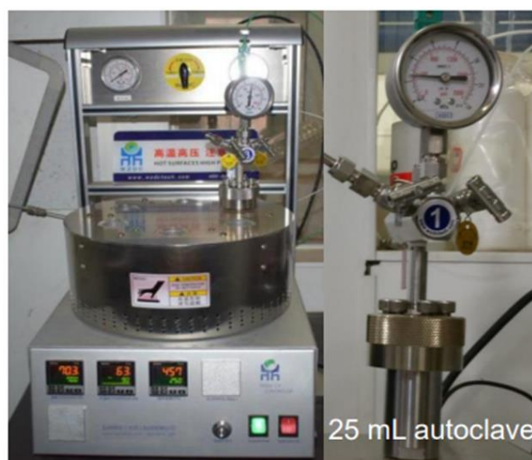
Figure S2. 25-mL autoclaves (Wuzhou Dingchuang (Beijing) Technology Co., Ltd.)
