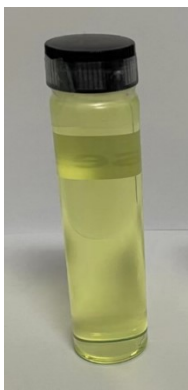
Fig. S4 Bio-oil photography (Reaction condition: 1.0 MPa H 2 , reaction temperature 280 °C, 6h, WHSV=2 h -1 , cyclopentanone, Cu/Al 2 O 3 -500b).
