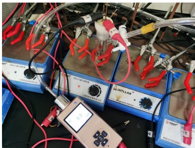
Figure S2 H 2 detection experiment by a H 2 detector
