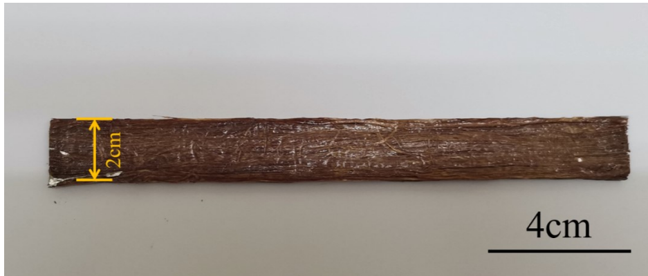
Fig. S13. Photograph of the CMDDB-0.5 of a large scale sample (16 cm in length, 2cm in width).
