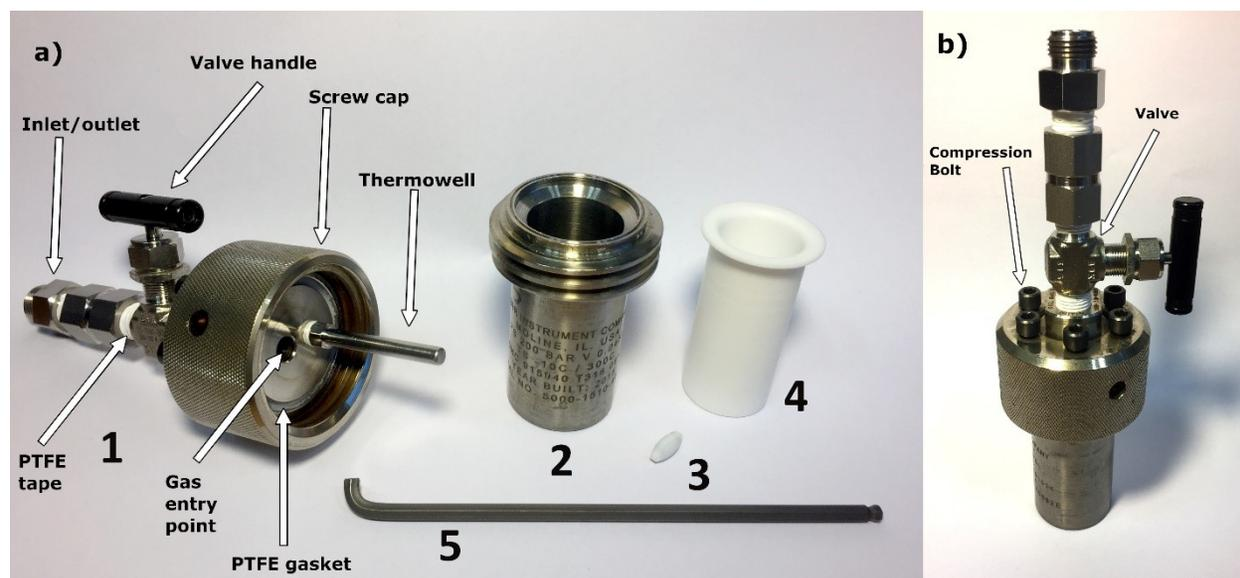
a) Parts of a pressure vessel: 1 – vessel head, 2 – 45 mL reaction well, 3 – magnetic stirring bar, 4 – 30 mL PTFE inlay, 5 – hex key for fastening bolts; b) assembled pressure vessel.
