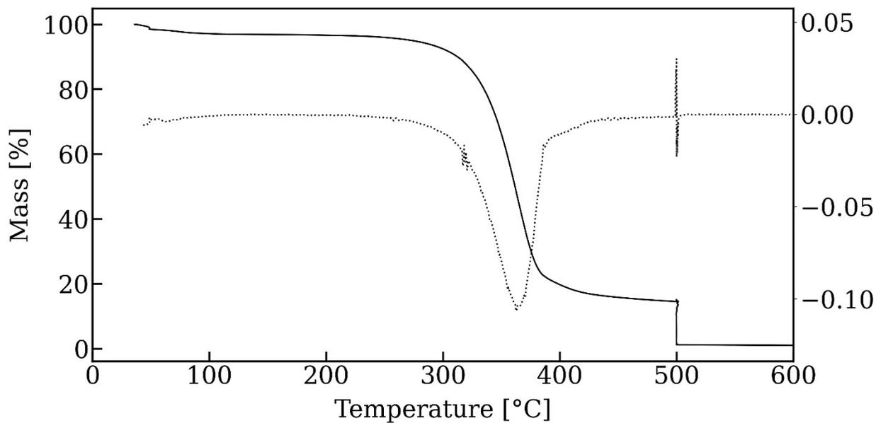
**TGA Spectra of Leftover Fabric from Cotton From Solvolysis in Laboratory Air (Top) and Nitrogen Atmosphere (Bottom)**
