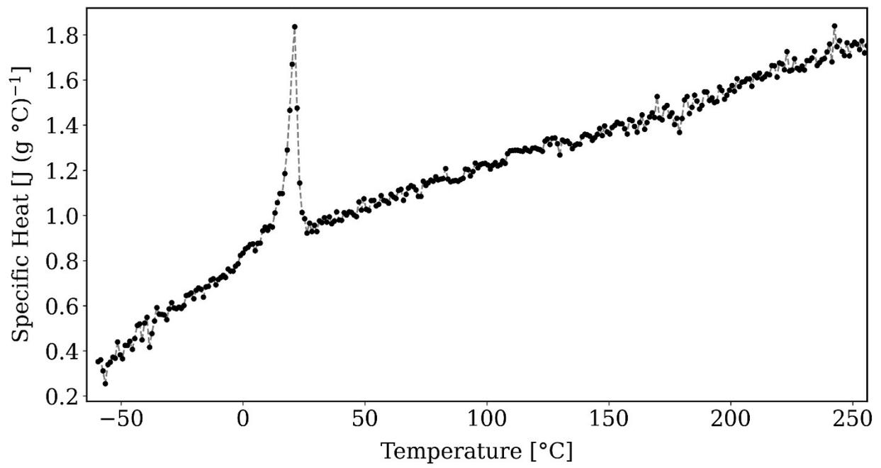
**DSC of Leftover Fabric from Tights with Two Heating-Cooling Cycles (top) and DSC StepScan (bottom)**
