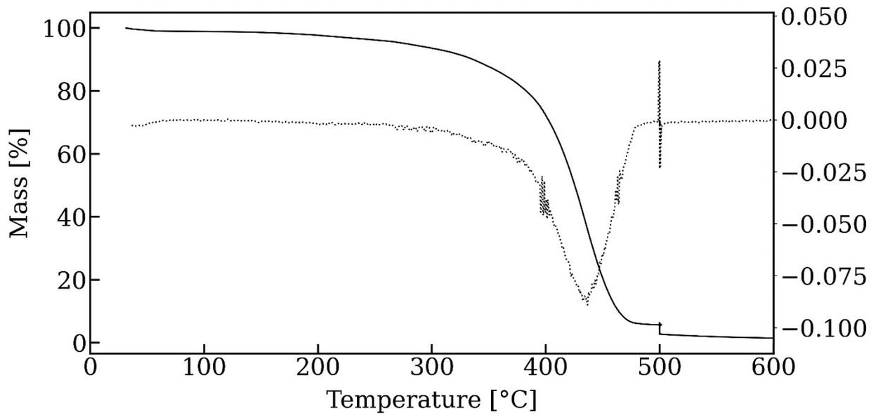
TGA Spectra of Leftover Fabric from Tights From Solvolysis in Laboratory Air (Top) and Nitrogen Atmosphere (Bottom)
