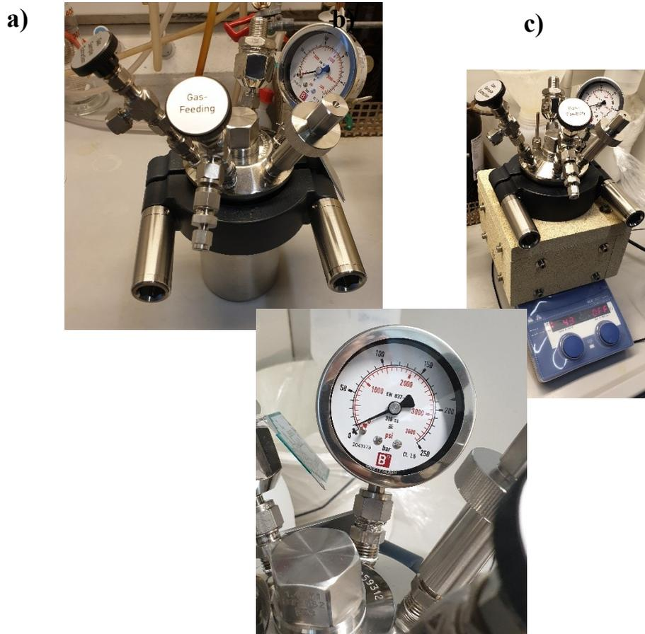
a) Assembled autoclave. b) Autoclave in heating block on stirring plate. c) Manometer for pressure read-out.
