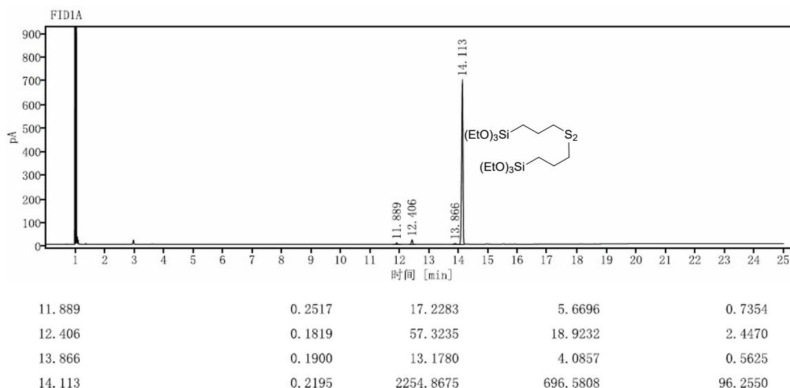
Fig.4 GC spectra of bis(triethoxysilylpropyl) disulfide (96.3% purity)
