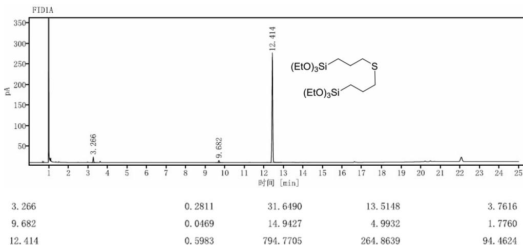
Fig.3 GC spectra of bis(triethoxysilylpropyl) sulfide (94.5% purity)
