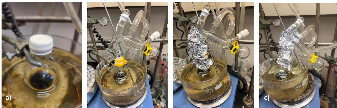
Figure 2. a) After thioester formation, with addition of alcohol and EtOAc; b-1) distillation set up; b-2) with foil added; c) with distillate collected
