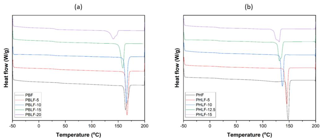
**Figure S22.** DSC heating traces of the polyesters in the PBLF (a) and PHLF (b) series of polyesters after annealing at approx. 10-15 °C below  $T_m$  for 4 h.
