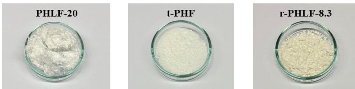
**Figure S32.** Photographic images of initial PHLF-20, t-PHF and r-PHLF-8.3 obtained after the repolymerization of t-PHF.
