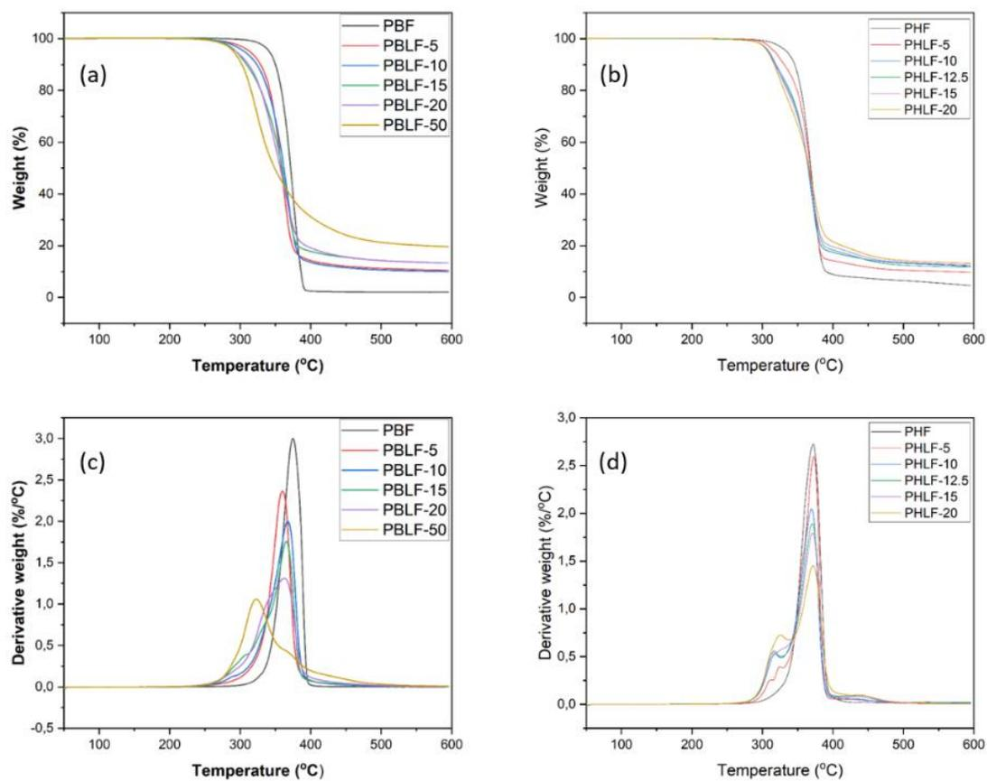
**Figure S19.** TGA thermograms and corresponding first derivative curves of the PBLF (a and c) and PHLF (b and d) series of copolyesters recorded under nitrogen atmosphere.
