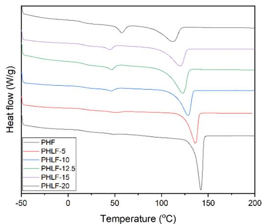
**Figure S21.** DSC heating traces of the polyesters in the PHLF series after storage at room temperature for 2 weeks.
