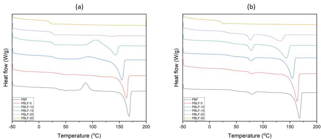
**Figure S20.** DSC heating traces of the polyesters in the PBLF series after storage at room temperature for 2 weeks (a) and at 50 °C during 40 h (b).
