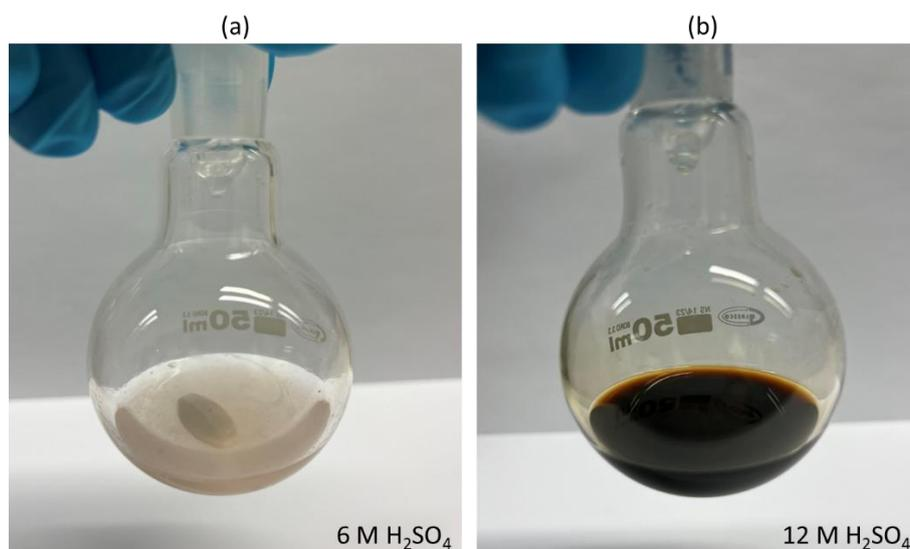
**Figure S30.** Photographs showing the reaction mixtures after the hydrolysis PHLF-20 in 6 M (a) and 12 M (b) aq.  $\text{H}_2\text{SO}_4$  at 85 °C after 24 h.
