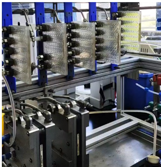
Figure SI2 Real picture of seven reactor plates in series
