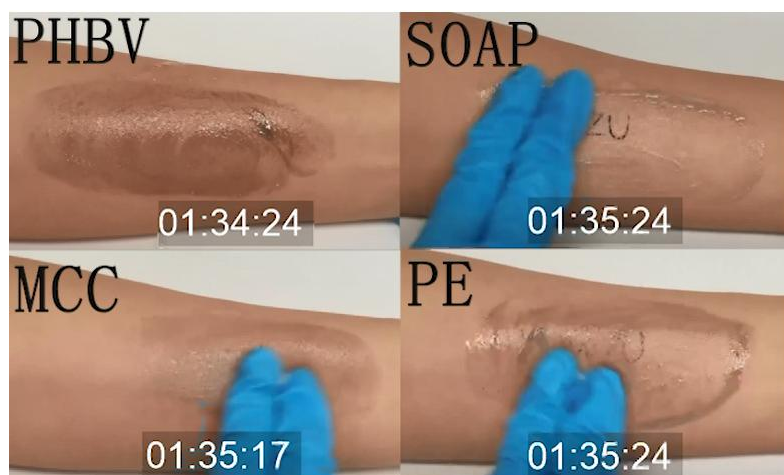
Figure S12. The cleaning image from cleansing movie when the contaminant was completely removed by PHBV microbeads.
