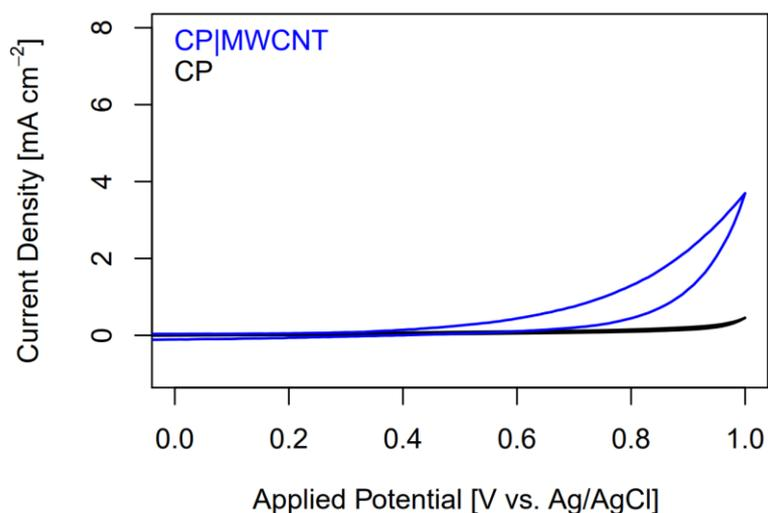
**Figure S9. Optimisation of electrooxidation conditions (blank).** Cyclic voltammetry of CP|MWCNT and CP. Reaction conditions: 0.1 M Na<sub>2</sub>CO<sub>3</sub> in 1:1 MeCN:H<sub>2</sub>O; -0.2 to +1 V vs. Ag/AgCl forward and backward scan; 50 mV s<sup>-1</sup> CE: Pt foil, RE: Ag/AgCl, room temperature.
