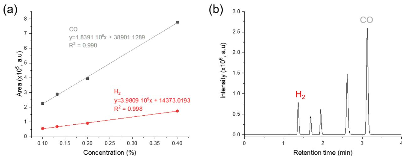
**Figure S22. H<sub>2</sub> and CO quantification.** (a) Calibration curve for H<sub>2</sub> (red) and CO (grey) quantification, and (b) spectra of H<sub>2</sub> (red) and CO (grey) at different concentrations obtained using gas chromatography.
