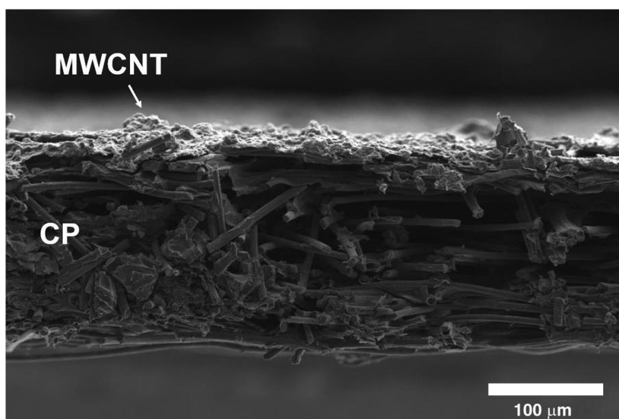
**Figure S8. Scanning electron microscopy of anode.** Scanning electron microscopy image of the cross section of CP|MWCNT.
