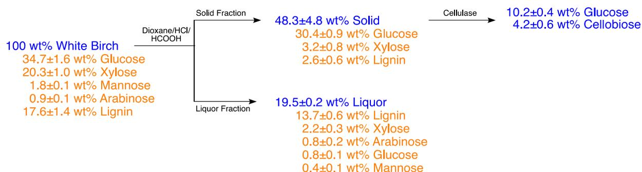
**Figure S1. Fractioning of lignocellulose into solid and liquid fractions.** Fractioning of Lignocellulose (white Birch) into a predominant cellulose and lignin containing fractions, and their composition with respect to (wrt) the isolated fractions (top) and white birch (bottom). Cellulose based solid fraction was further incubated with cellulase to generate a soluble sugar (glucose and cellobiose) solution.
