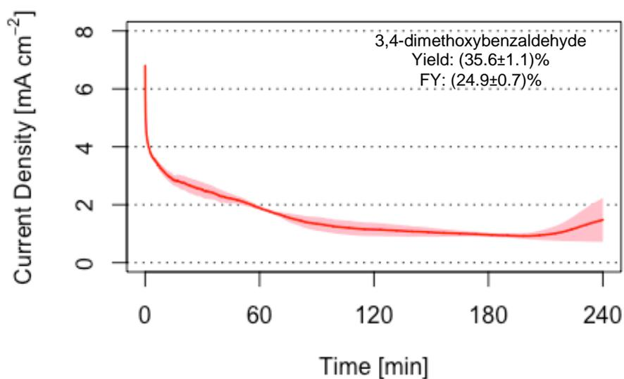
**Figure S11. Chronoamperometry of optimised anode with lignin substrate model in three-electrode setup.** Chronoamperometry trace of lignin model substrate with CP|MWCNT to form 3,4-dimethoxybenzaldehyde. The shaded area represents the standard deviation. Reaction conditions: CA: 0.1 M Na<sub>2</sub>CO<sub>3</sub>, 0.01 M Lignin Model in 1:1 MeCN:H<sub>2</sub>O; +1 V vs. Ag/AgCl; 4 h WE: CP|MWCNT, CE: Pt foil, RE: Ag/AgCl, room temperature.
