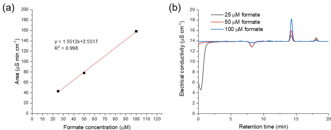
**Figure S23. Formate quantification.** (a) Calibration curve for formate quantification, and (b) spectra of formate at different concentrations obtained from ion chromatography (retention time 14.2 min).
