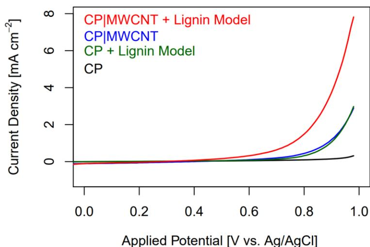
**Figure S10. Optimisation of electrooxidation conditions.** Cyclic voltammetry of CP|MWCNT and CP with and without the lignin model substrate (0.01 M). Reaction conditions: 0.1 M Na<sub>2</sub>CO<sub>3</sub> in 1:1 MeCN:H<sub>2</sub>O; -0.2 to +1 V vs. Ag/AgCl forward and backward scan; 50 mV s<sup>-1</sup> CE: Pt foil, RE: Ag/AgCl, room temperature.
