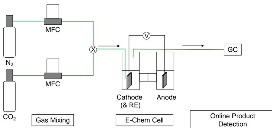
**Figure S6. Flow setup for variable concentration CO<sub>2</sub> electrocatalysis.** Scheme for CO<sub>2</sub> electrocatalysis under flow by controlling the gas composition with mass flow controllers purging the gas through the anolyte followed by online-GC analysis to detect H<sub>2</sub> and CO.<sup>1</sup>
