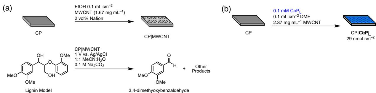
**Figure S5. Electrode preparation.** (a) Preparation of CP|MWCNT electrode and electrocatalytic lignin model substrate oxidation. (b) Preparation of CP|CoP<sub>L</sub> electrode for CO<sub>2</sub> electroreduction to CO.
