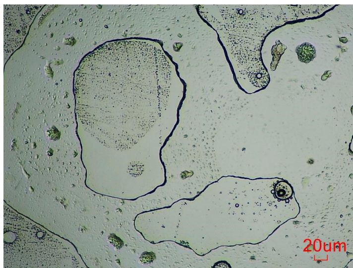
Figure S31: Microscopic image of olive oil in water emulsions without the use of any additive taken after leaving the emulsions for 24 h.
