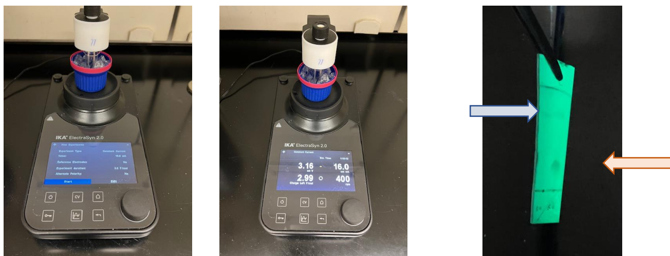
Figure S5. Electrochemical defluorinative carboxylation apparatus set up and TLC confirmation. (Left) The reaction vial is maintained at 0°C via sustaining an ice bath in large, standard beaker cap. The parameters are set to constant current 16mA with 3.0F/mol of 0.25 mmol of substrate. No reference electrode is used. (Centre) The electrochemical experiment running as normal with the voltage and duration displayed. (Right) Thin layer chromatography (TLC) was conducted with the reaction (red arrow) compared to the starting material (blue arrow). This was viewed under UV light of 254 nm.
