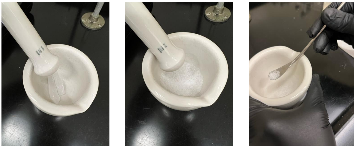
Figure S3. Addition of dry ice methodology. (Left) A common mortar and pestle is all that is required to grind the large chunks of dry ice into small pellets to be added into the reaction vial. (Centre) Within seconds, the large chunks of dry ice are grinded into small pellets of dry ice. (Right) A small spatula full is all that is required to be added into the reaction vial at the start of the reaction and every 10-15 minutes intervals afterwards until completion.
