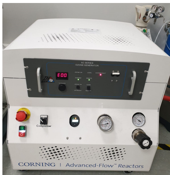
Figure S2: Picture of the exterior of the ozone dosing line from Corning®
