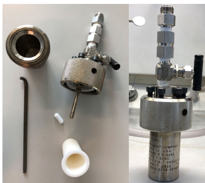
Figure S2. 45 mL steel autoclave with 30 mL PTFE inlay.
