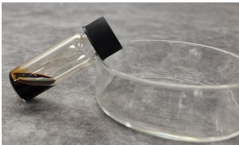
**Fig S3.** Mixture of oligomeric lignin and thymol at a mass ratio of 1:2 at room temperature, demonstrating the liquid appearance of the mixture.
