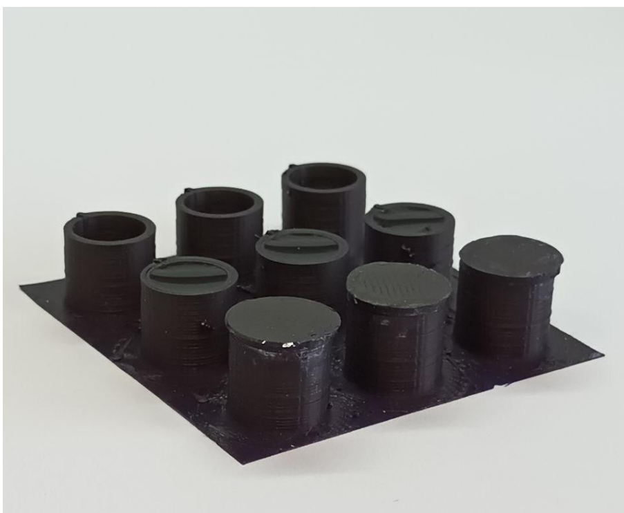
Figure S40. Photo of sealing of filled vials with caps using glue; the glue was made from the same plastic and an appropriate solvent.
