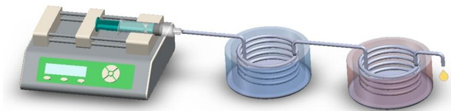
**Figure S1.** Continuous flow platform of *Flow\_2* for polyamide synthesis
