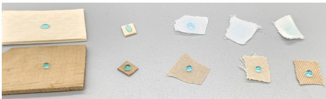
Fig.S8 The images of water droplet on pristine substrate (First line from left to right: wood, straw and composite fabric (65%polyester-35%cotton, 80%polyester-20%cotton, and 100%cotton)) and corresponding images on modified substrate in second line after the deposition of FLP/Fe.
