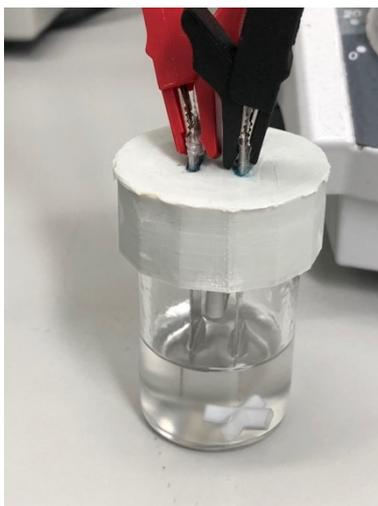
**Figure S1:** Electrochemical setup for batch electrolysis in an undivided cell using a glass vial with a 3D printed cap.
